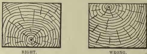
Fig. 105. Right and Wrong Method of Laying Ties.
