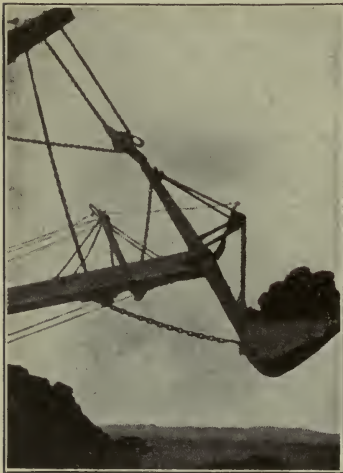
Fig. 42. Dipper and Dipper Handle of Walking Scoop Dredge
