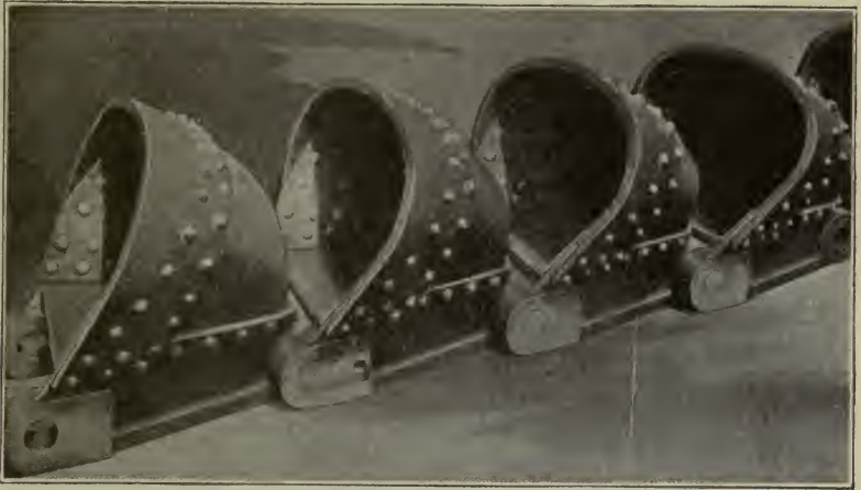
Fig. 55. Section of Chain Used on Ladder Dredge
