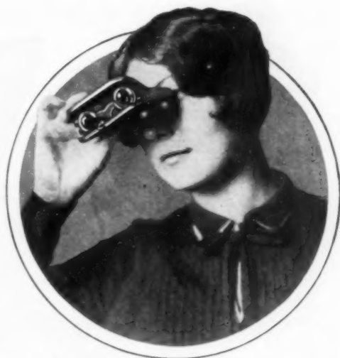
Glasses Opened to Expose the Lenses; When Folded, They Can Be Slipped into the Pocket
