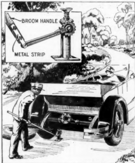
Broomstick Bolted to Jack Handle Gives Motorist Considerable Leverage
