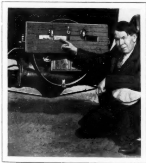
Motion Sign at Rear of Auto; a Reel with Words on It Turns as the Car Proceeds
