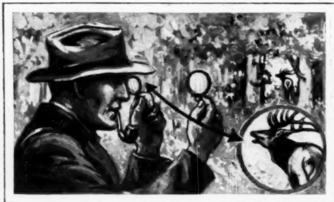
Drawing of the Lenses in Actual Use; Focusing Is Accomplished by Moving the Larger Glass Backward or Forward
