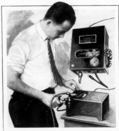
Testing Spark Plugs under Pressure, to Reveal Defects That Might Appear in Actual Operation
