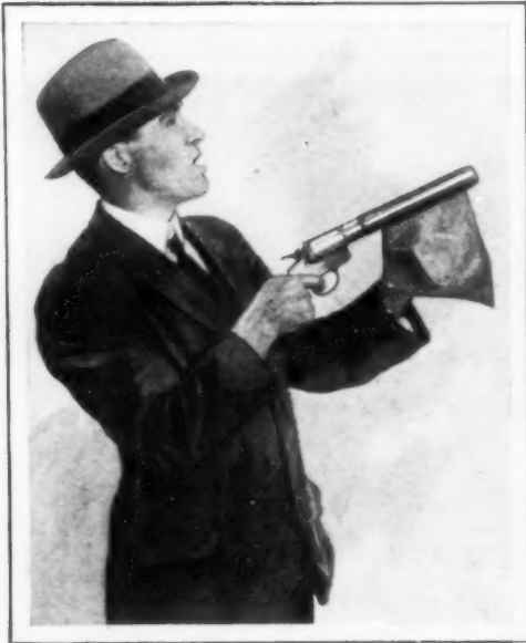
Shooting Life Line from the Pistol; the Flap Protects User's Hands from Powder Flash
