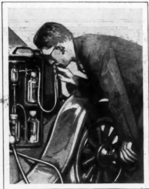
Testing Auto's Exhaust Fumes, to Determine if the Carburetor Has Been Adjusted Properly
