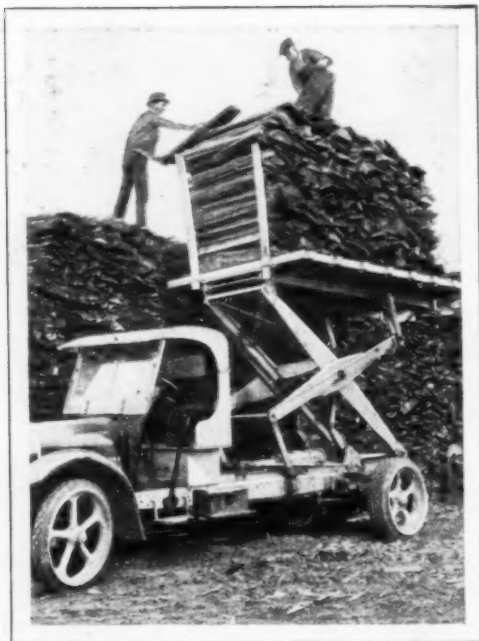
Eliminating Laborious Lifting; the Elevated Truck Body Extended to Simplify Task of Stacking Wood
