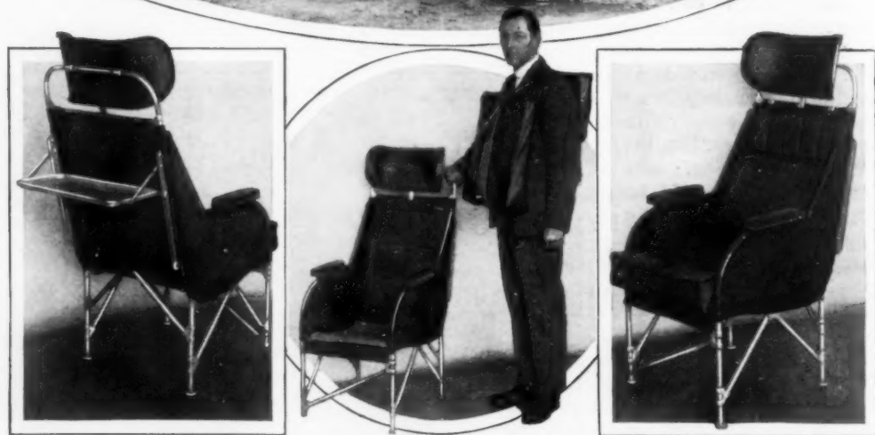
Passengers Who Ride on Air Cushions in New British Liners Can Wear the Seats as Life Preservers; at Left, Food Tray on Back of Seat; Other Views, the Life-Preserver Cushions
