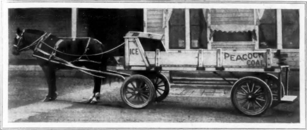
Using Discarded Auto Wheels and Axles on a Wagon Makes It Easy-Riding and Noiseless
