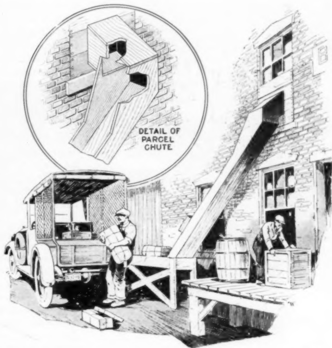
Handy Wooden Chute Conveys Parcels from Second-Floor Shipping Room to a Loading Platform Below.
