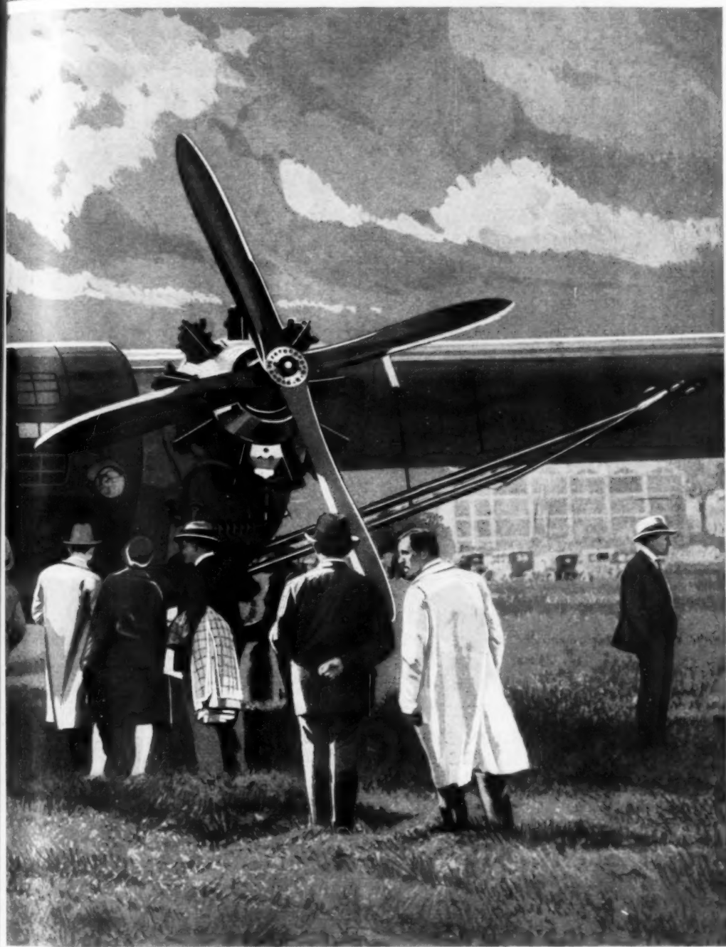
Instead of the Usual Fuselage, the Crew and Bombs Are Housed in What Is Really a Thickened Section of the Wing; the Craft Weighs Five and a Half Tons and Makes 100 Miles an Hour
