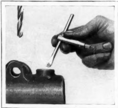
Handle of Lathe Chuck Wrench Ground Down to Spoon Shape Adds to Its Usefulness
