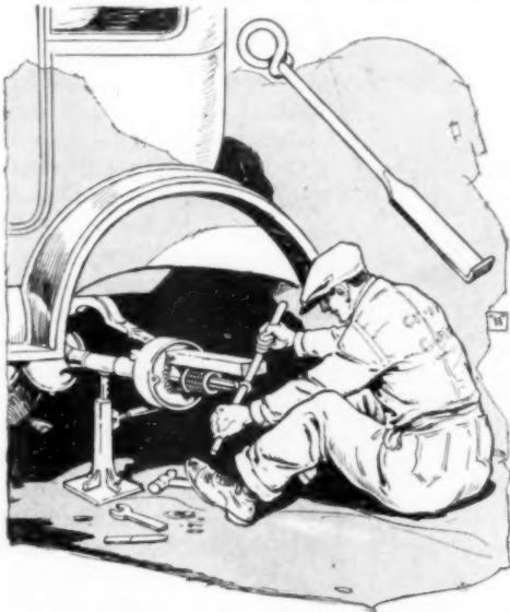
Roller Bearings on Ford Axles Can Readily Be Removed with This Simple Tool
