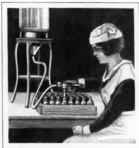
Suitable for Home or Cannery Use; a Bottle Filler with Control Valve to Eliminate Spilling
