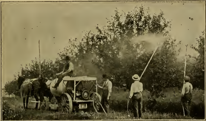
Fig. 60.—One of the many types of sprayers with power from a gasoline engine.
