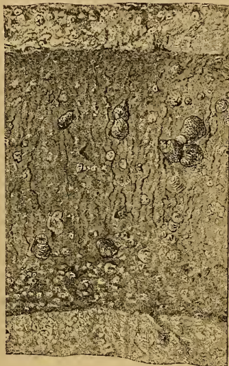
FIG. 1.—LOWER SIDE OF TILE EXPOSED JULY 9-AUG. 2. (TWO-THIRDS NATURAL SIZE.)
