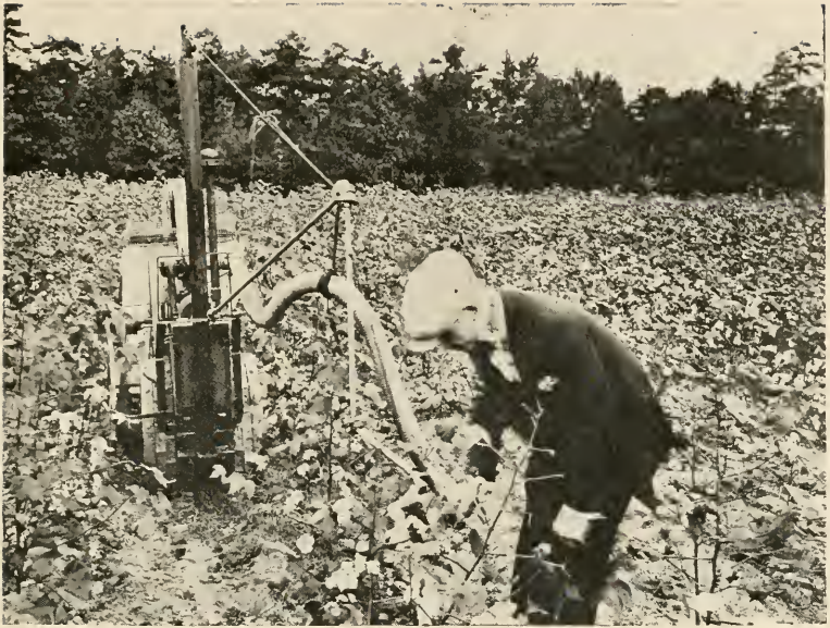
Stukenberg Single Head Cotton Picking Machine Attached to a Small Beeman Garden Tractor
