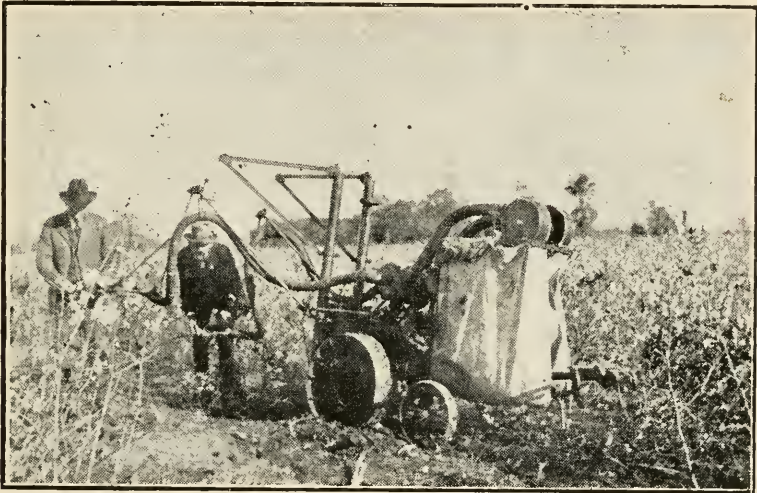
Stukenberg Double Head Cotton Picking Machine Attached to a Small Beeman Garden Tractor
