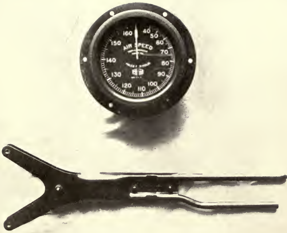
AIR SPEED INDICATOR--DIAL AND HEAD
