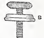
Fig. 4.—Binding Screw (A) and Adjusting Screw (B).
