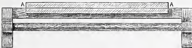
Fig. 2.—Towel Rail: Front Elevation (A, A, Flap) and Side Elevation. (Scale, 2 in. to 1 ft.)
