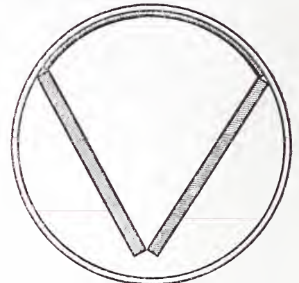
Fig. 3.—Plan of Tube at Object End, with Object Box Removed (full size).
