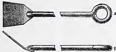
Fig. 3.—Spoon for Transferring Sections to Slide in—Front View (A) and Side View (B).
