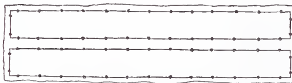
Fig. 30.—Winding Strips Lined out and Centre-popped on piece of Steel Plate.
