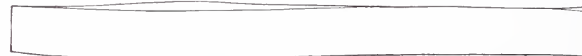
Fig. 29.—Another Example of Trial of Straightedge against Line marked from own Edge.
