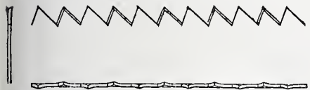
Fig. 10.—Teeth of Hand Saw for Cross Cutting.
