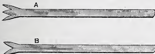
Fig. 5.—Forks for Marking for Bridge Pins: actual size. A, Trichord; B, Bichord.
