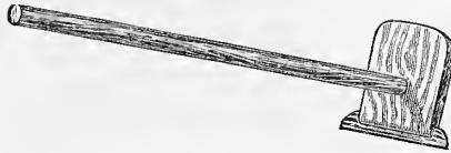
Fig. 1.—Hammer generally used by Cabinet Makers in Veneering. A Home-made Tool.
