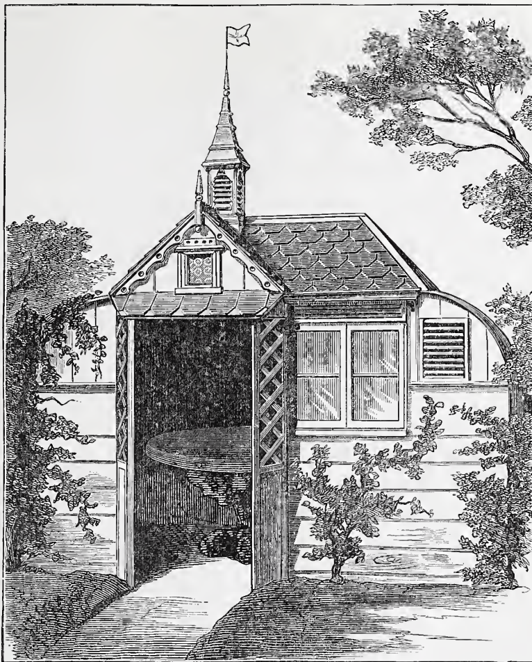
Fig. 1.—Summer-House roofed with Linoleum Tiling.
