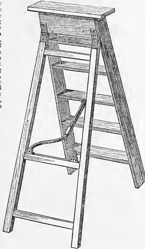
Fig. 1.—Step Ladder Opened and Locked for Use.
