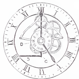
Electric Time Alarm. Fig. 1.—D, is the Disc full size; S, the Spring; C, the Catch. Fig. 2.—Disc fitted on Clock.
