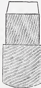
Fig. 23 B. — End View of Round-Soled Plane.
