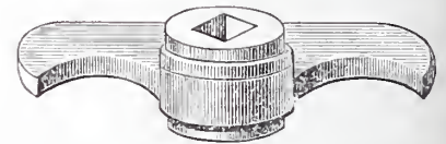
Fig. 8.—Follower in Mortise Lock, showing Form, etc.
