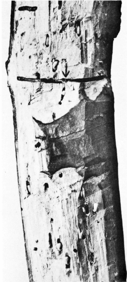
Figure 9.—Piece of hickory with the bark and a little of the wood removed, revealing tunnel of an adult powder-post beetle ( Xylobiops basilaris (Say)). Entrance hole is shown at tip of arrow, and the gallery is seen extending on each side. Larvae, pupae, and emerging adults are shown in their cells. Natural size.
