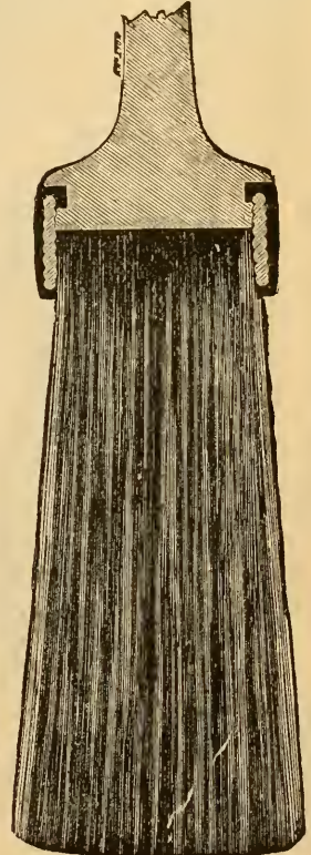
Sectional view of Round Paint Brush cut in two.
