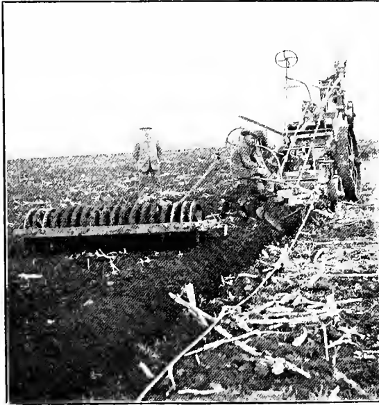
FIG. 153.—Steam-ploughing and subsoil packing the land at Vereeniging; double engine system. (Courtesy of Messrs. John Fowler & Co.)
