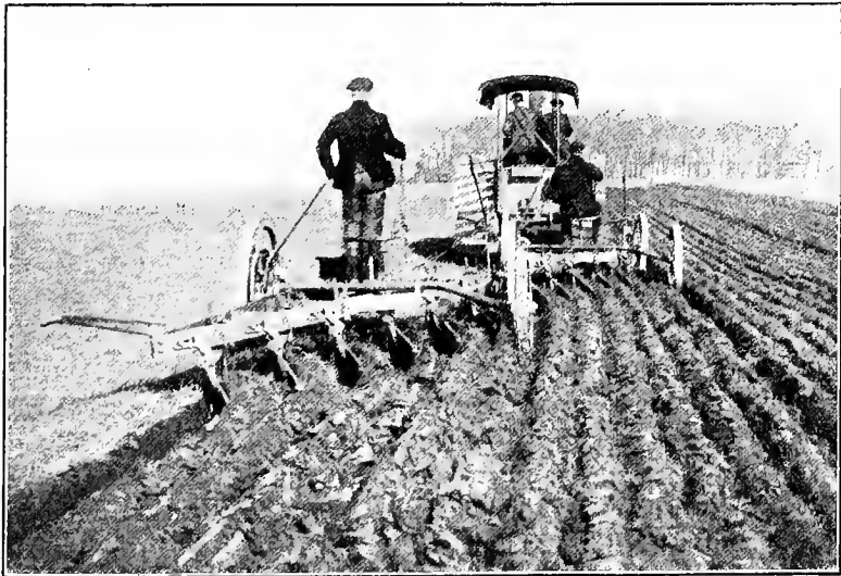
FIG. 131.—Deep ploughing by steam, 12 furrows at a time by direct traction.
