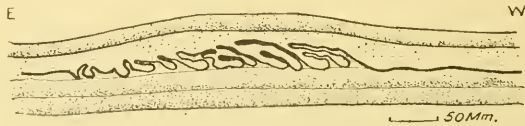
FIG. 39.—Detail of clay layer erumped by the current, from fig. 38, to show how the layer was carried along by the friction of a current from the west.
