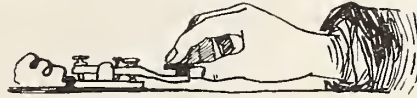
Figure 2. This illustrates the correct position of the hand when sending. The wrist should not touch the table, and the heavier muscles of the forearm should do the work, the finer touches being made by the more delicate muscles of the wrist and fingers.
