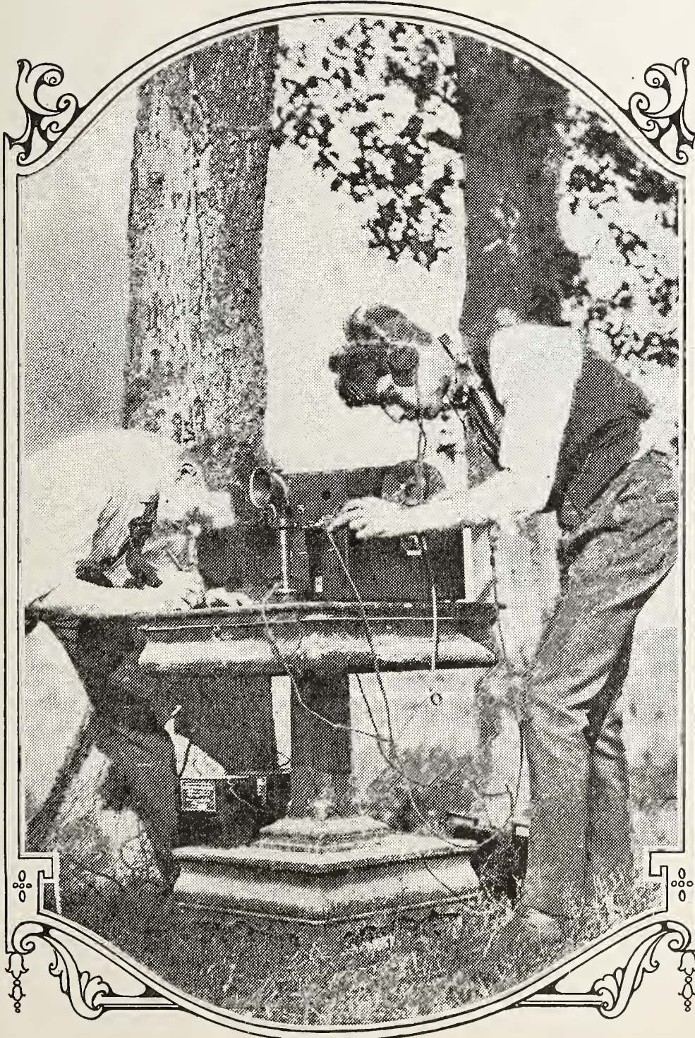
During the war experiments proved that it is possible to use trees instead of the usual antennae for wireless receiving outfits. These two Atlantic coast boys are giving the trees a chance to speak. Press Illustrating Service Photo
