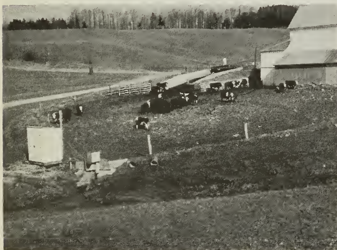
FIG. C-7.—Animal waste from a beef cattle barnlot is gaged and sampled.
