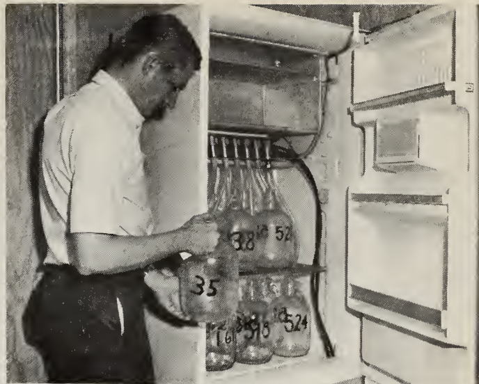
FIG. C-4.—Runoff samples in field refrigerator are obtained for determining pollutants in water and on soil particles washed off farmland.
