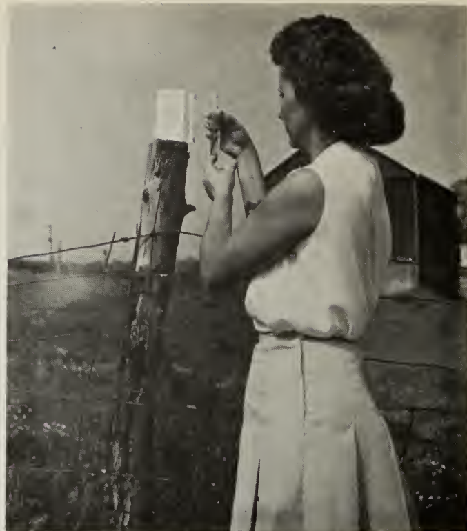
FIG. B-3.—Cooperative observer reading rain depth in glass tube.
