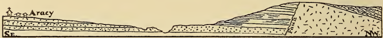
FIG. 5. Section about three kilometers long northwest from Aracy, showing the faulted Estancia beds against granites.
