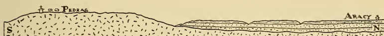
FIG. 9. North-south section from the village of Pedras to Aracy showing the Estancia beds overlying granites.
