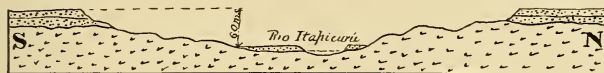
FIG. 10. North-south section across Rio Itapicuru at Engenho Brauna, 12 kilometers north of Timbó, State of Bahia. Mesozoic sediments forming the plateau rest upon granites, gneisses, and schists.
