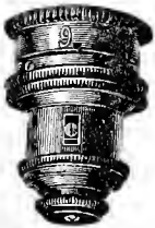
FIG. 19. Achromatic objective with correcting apparatus.
