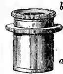
FIG. 54. Polarizer. The tube a fitted into the stage; b , convex lens of flint-glass.
