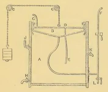
A, square; B, the OCTUPLE or double cover; C, C, pulleys and chain, by which it is lowered or raised; D, a tube through which the beer drains and passes to near the bottom of the tun through hose E; F, ingress water-pipe to take a flexible tube; G, egress water-pipe; the bent arrows show the direction the yeast takes; H, racking cock; J, thermometer; K, sample cock; L, cock by which the OCTUPLE is emptied of water.
