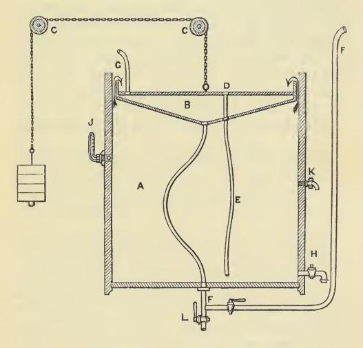
A, square; B, the Octuple or double cover; C, C, pulleys and chain, by which it is lowered or raised; D, one of four tubes through which the beer drains and passes to the bottom of the tun through hose E; F, ingress water-pipe to take a flexible tube; G, egress water-pipe; the bent arrows shew the direction the yeast takes; H, racking cock; J, thermometer; K, sample cock; L, cock by which the Octuple is emptied of water.
