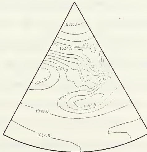
Figure 5.6f. Sea-level pressure contours for nonlinear Experiment 1 at 42 h. Contour interval is 2.5 mb. Domain is a 45^\circ sector of the globe with cyclic continuity at the east and west boundaries.
