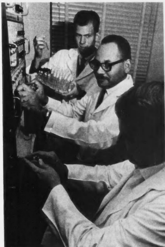
Chemist Patrick Crowe (right) and research chemist Alonza Hayden (center) use a gas chromatograph to test a meat sample. The chemists were freed for purely professional work when the Market Quality Research Division began hiring University of Maryland students such as Douglas Eilers (left) as part-time assistants.
