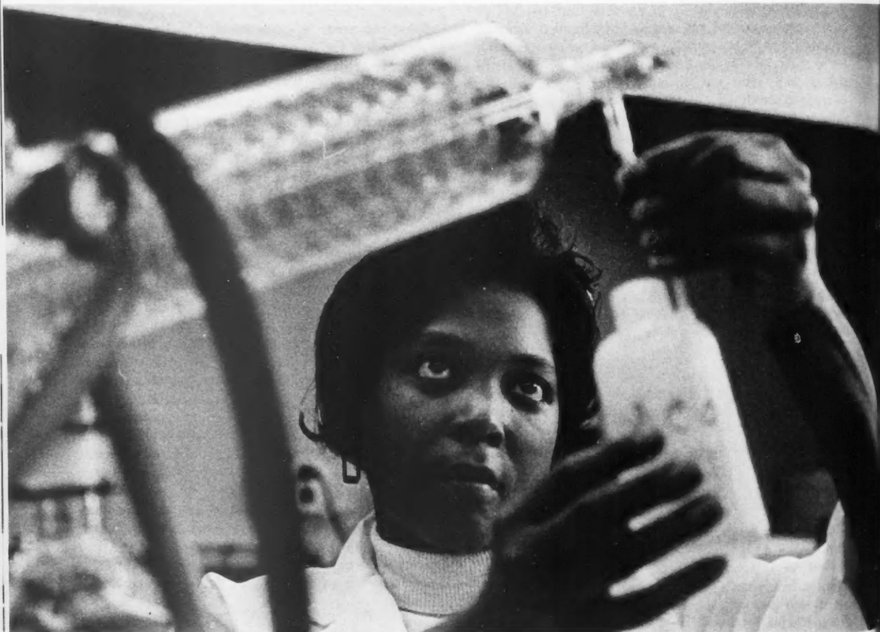
Mrs. Jacqueline Hall feeds methanol into a vacuum evaporator to identify different pigments in cherries. She is a laboratory helper in the Human Nutrition Research Division, Food Quality and Use Laboratory, Beltsville, Md.
