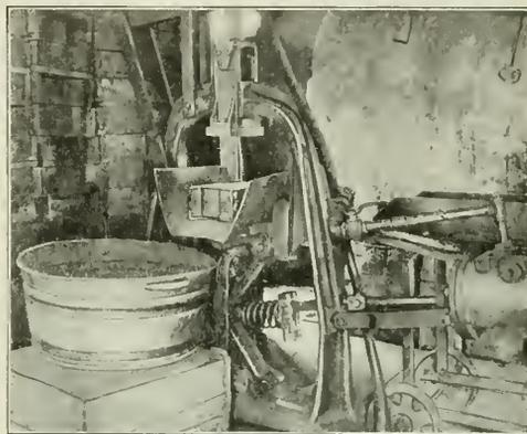
FIG. 5. HOME-MADE BRIQUETTING PRESS AT WEST END MILL
