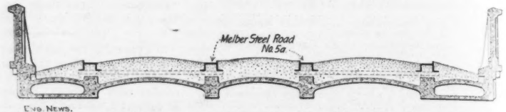
FIG. 5.—CROSS-SECTION OF CONCRETE BRIDGE WITH CONCRETE ARCH RIBS AND FLOOR ARCHES. F. Meiber, Pittsburg, Pa., Designer.
