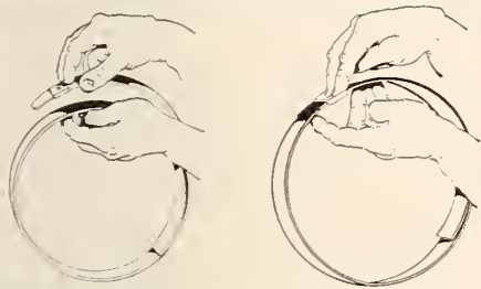
FIGURE 4 (left): A plastic reel band which uses a clip in place of the usual string for securing it about the reel; and FIGURE 5: The plastic reel band closed and secured by simply pressing down on the clip.
