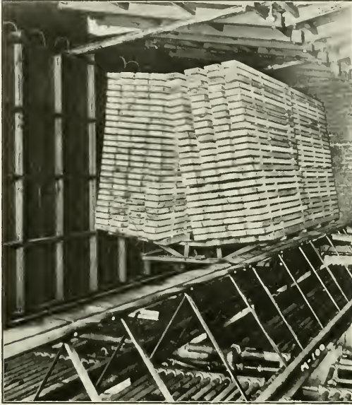
Interior of Humidity Controlled Dry Kiln
