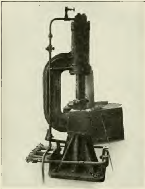
Pneumatic Hammer Used in Reclaiming Track Spikes
