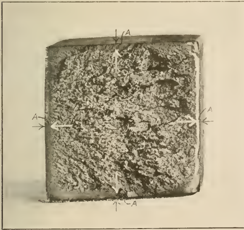
Fig. 2—Sample Bar Showing the Depth A of the Casehardening (Twice Actual Size)
