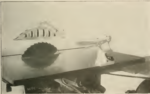
Fig. 2—Saw Guard Partially Raised
