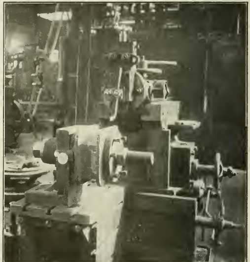
Finishing Rod Brass in Index Head on a Shaper
