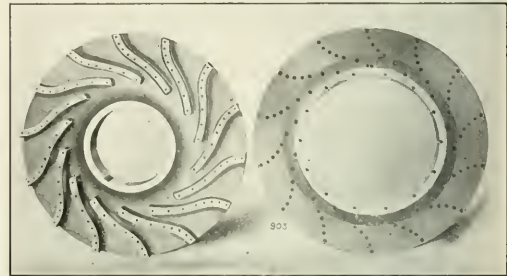
Impeller Disc and Side Plate of Multi-Stage Air Compressor Showing Method of Attaching Vanes
