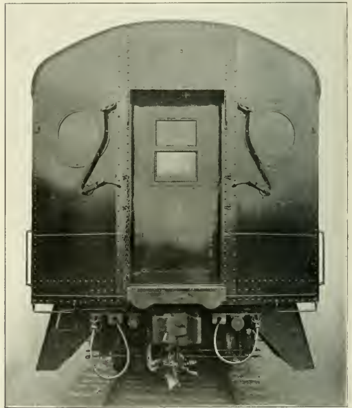
End View of the Long Island Trailer Showing the Permanent Jumpers
