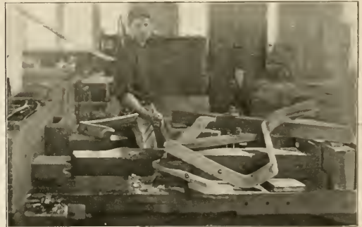
Fig. 14—Formers for Making Brake Mast Supports
