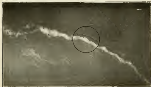
Fig. 1—Radiograph of Steel Casting Showing a Blow Hole Below the Surface. The Circle Shows Where the Button Was Removed
