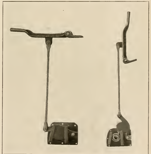
Brine Tank Drain Valve in Closed and Open Positions
