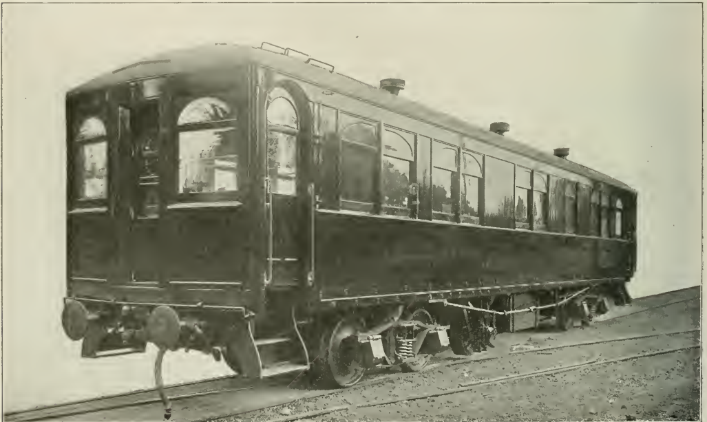
Dynamometer Car for the Japanese Government Railways; the Trucks Shown Are Temporary
