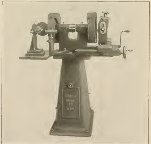
Chaser Grinder and Disc Sharpener for the Cutters of Roller Pipe Cutting Machines
