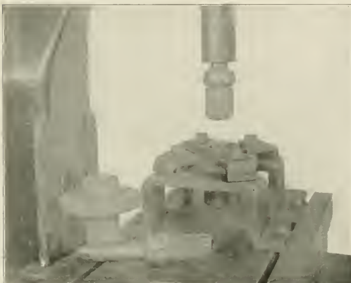
Finishing Valve Seat End of Tank Valve Casting
