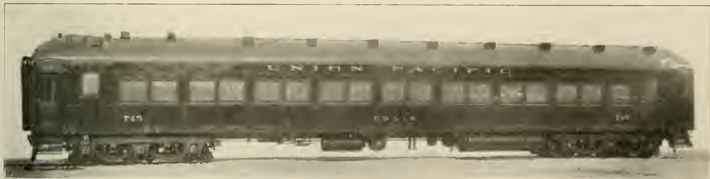
Reclining Chair Car of All-Steel Construction, Used on the Union Pacific
