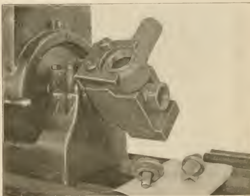
Chuck in Position for Finishing the Branch Pipe Connection
