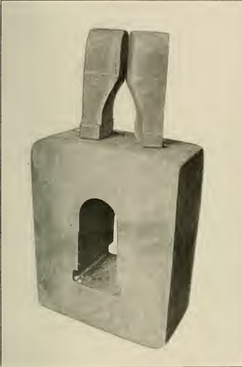
Fig. 2—Cup and Blocks for Forming Spring Hanger Shown in Fig. 1
