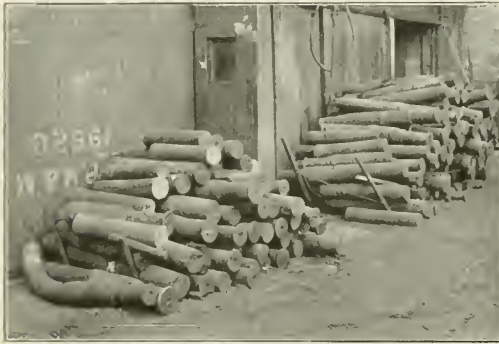
Fig. 4—Sheared Wrought Iron Axles Which Are to be Rolled into Refined Iron Bars
