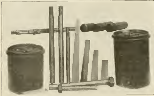
Cutter Heads, Blades and Gages for Adjusting the Heads; Hollow Gages for Testing Turned Bolts
