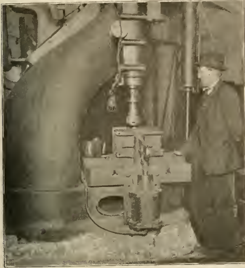
Old Car Wheel Boring Mill Converted for Boring Driving Boxes
