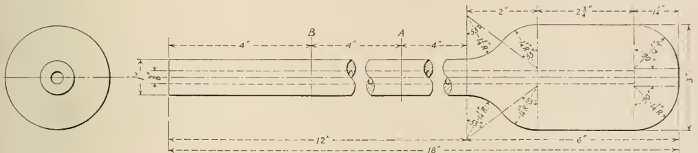
Fig. 1—Test Piece Used in Quenching Tests
