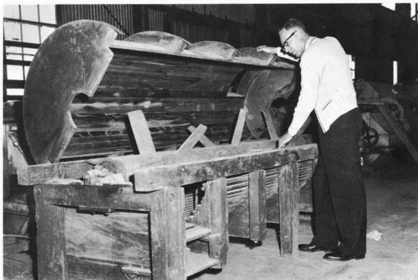
A seed cotton cleaner built of wood by a slave for the Blakley Plantation gin north of Vicksburg, Miss.
