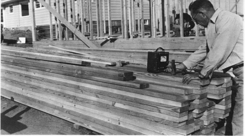
Moisture meters developed at the Forest Products Laboratory make it possible to determine whether lumber has been seasoned properly.
