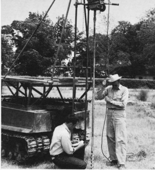
A power auger is used to get at the deeper layers of soil that influence the planning of irrigation.
