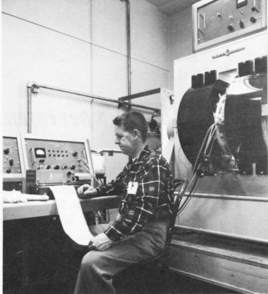
Nuclear magnetic resonance is used to identify flavor components of fruit and vegetables, determine radiation damage, and characterize complex molecules.
