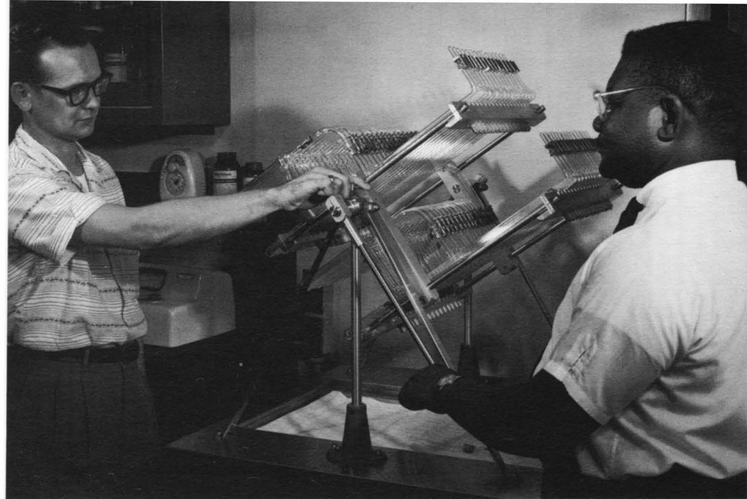
M. O. Bagby and T. L. Wilson, research chemists at the Northern Regional Research Laboratory in Peoria, Ill., operate an apparatus that separates complicated plant products into pure compounds.
