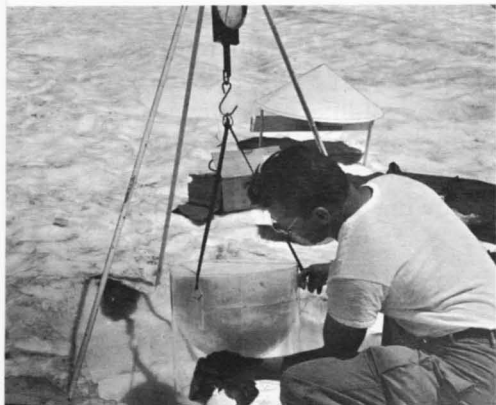
Measurements of evaporation on a summer snowfield. A plastic tank is set with its top level with the surrounding snow. A false bottom allows melt water to flow out of the snow. Repeated weighings give the loss by evaporation or gain by condensation.
