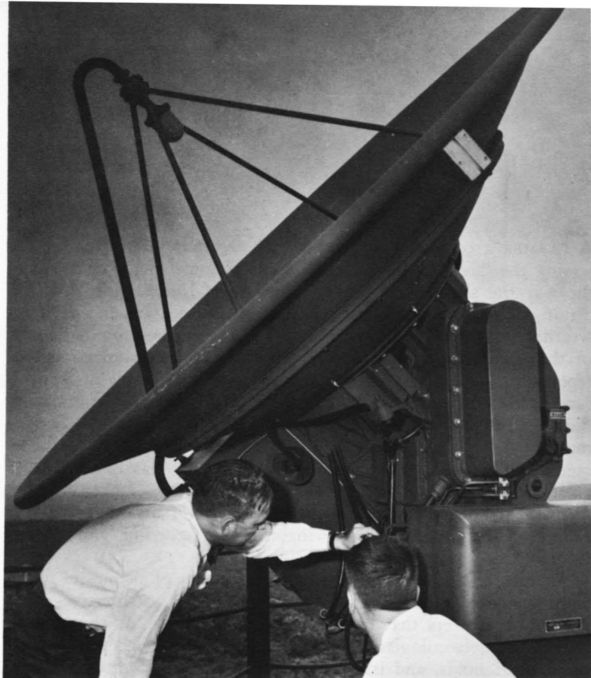
One of the radar antennae used in weather detection by the United States Weather Bureau, the Department of Commerce.
