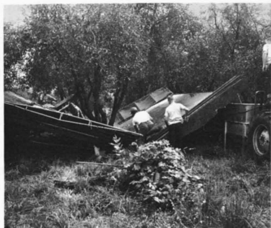
A boom-type shaker, collecting frames, and pallet tanks are used in harvesting tart cherries.
