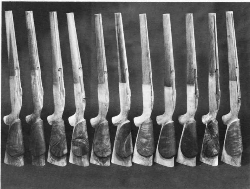
A new chemical seasoning process eliminates drying checks and splits and adds dimensional stability in these walnut gunstocks.
