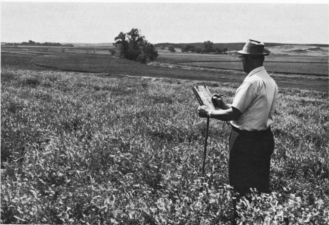
A soil scientist in Oklaboma has determined the kinds of soils and is sketching their boundaries on an aerial photograph.
