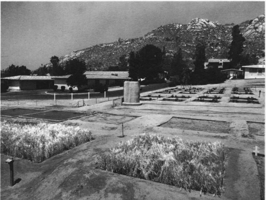
Small plots for testing the salt tolerance of plants at the United States Salinity Laboratory, Riverside, Calif.
