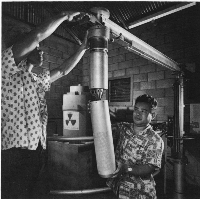
After attachment to the arm of the hoist, the cannister containing many thousands of pupae is inserted into the chamber in the lead cask, in the background of the photograph, which contains radioactive cobalt. Adult flies emerging from the treated pupae are sterile.
