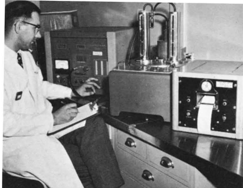
Edward C. Miller records results from a proportional flow counter at Beltsville to determine how birds metabolize certain nutrients that have been tagged with radioisotopes.
