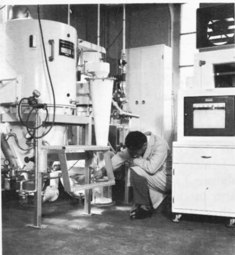
A spray drier is used in tests to develop new or improved egg products.
