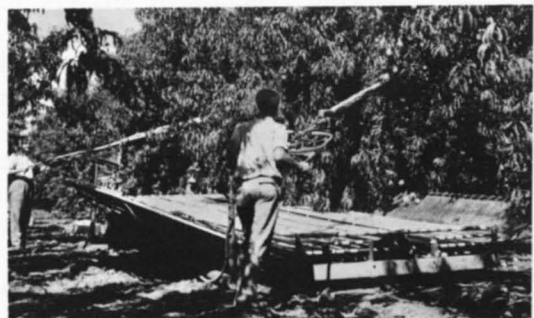
This is a bazooka-type impact harvester used in picking clingstone peaches.
