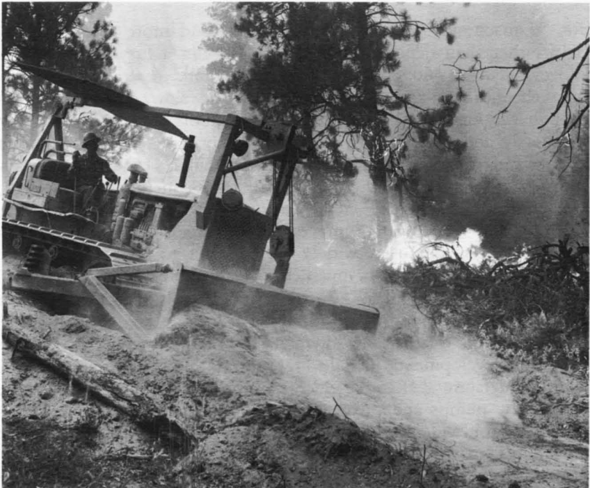
A tractor makes a fire lane near the edge of a fire on the Boise National Forest in Idaho.
