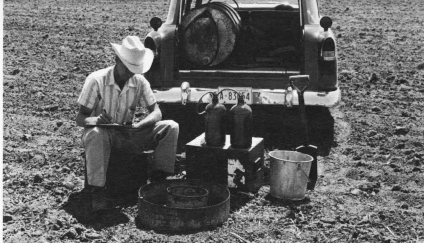
A device for determining how fast water enters the soil. This knowledge is necessary for planning irrigation or terraces.
