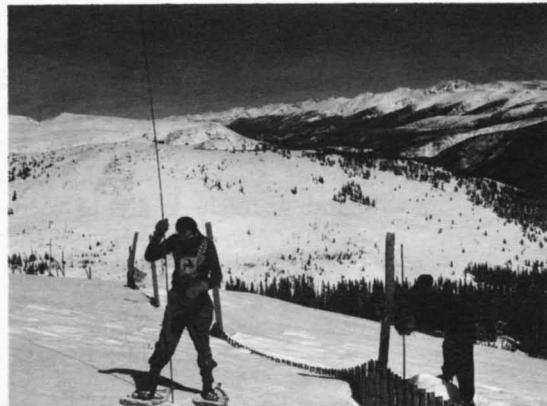
Probing in a fence-test area to measure the depth of trapped snow. Drifted snow packs to a higher density than freshly fallen snow.
