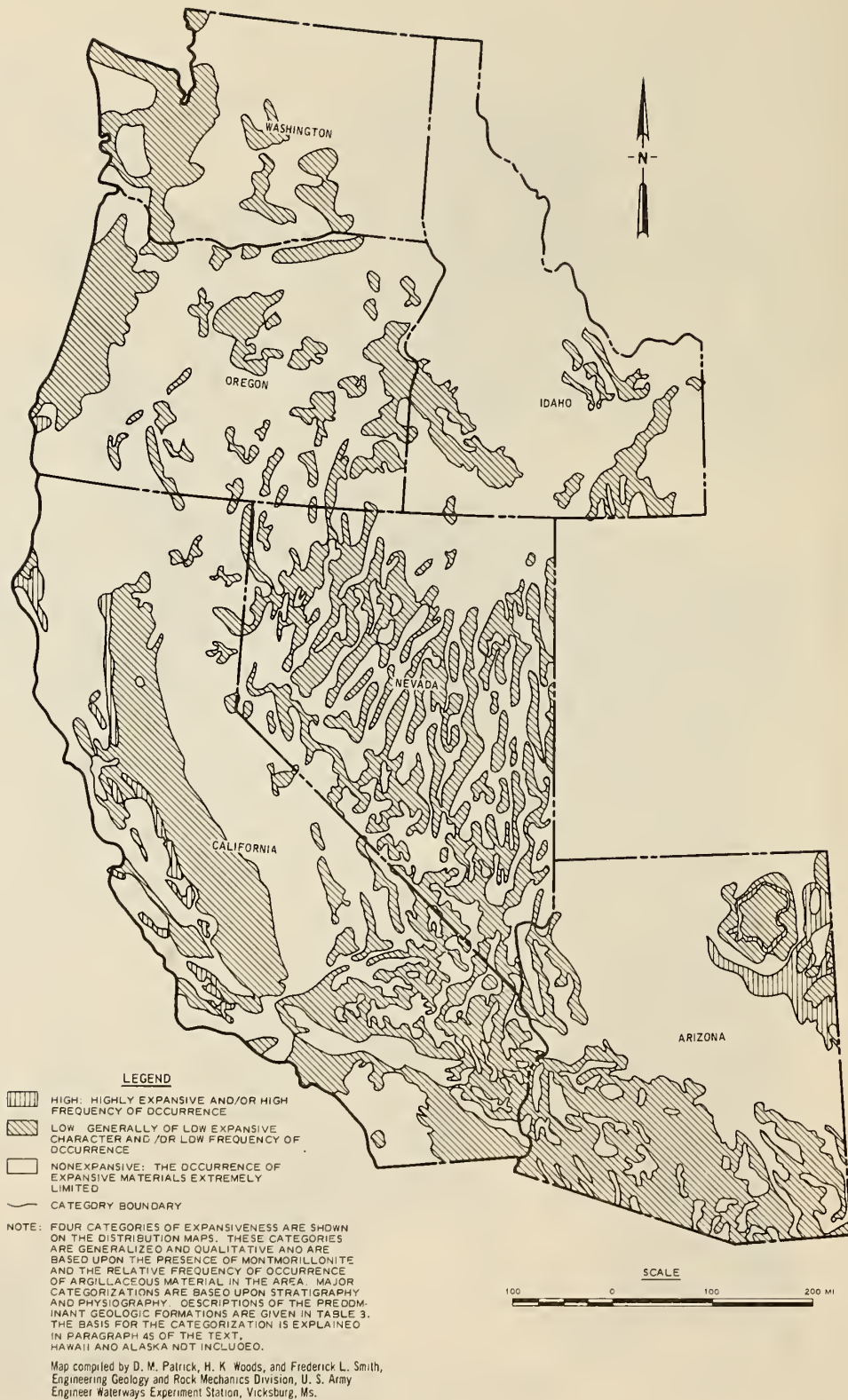
Figure 9. Distribution of potentially expansive materials in the United States; FHWA Regions 9 and 10
