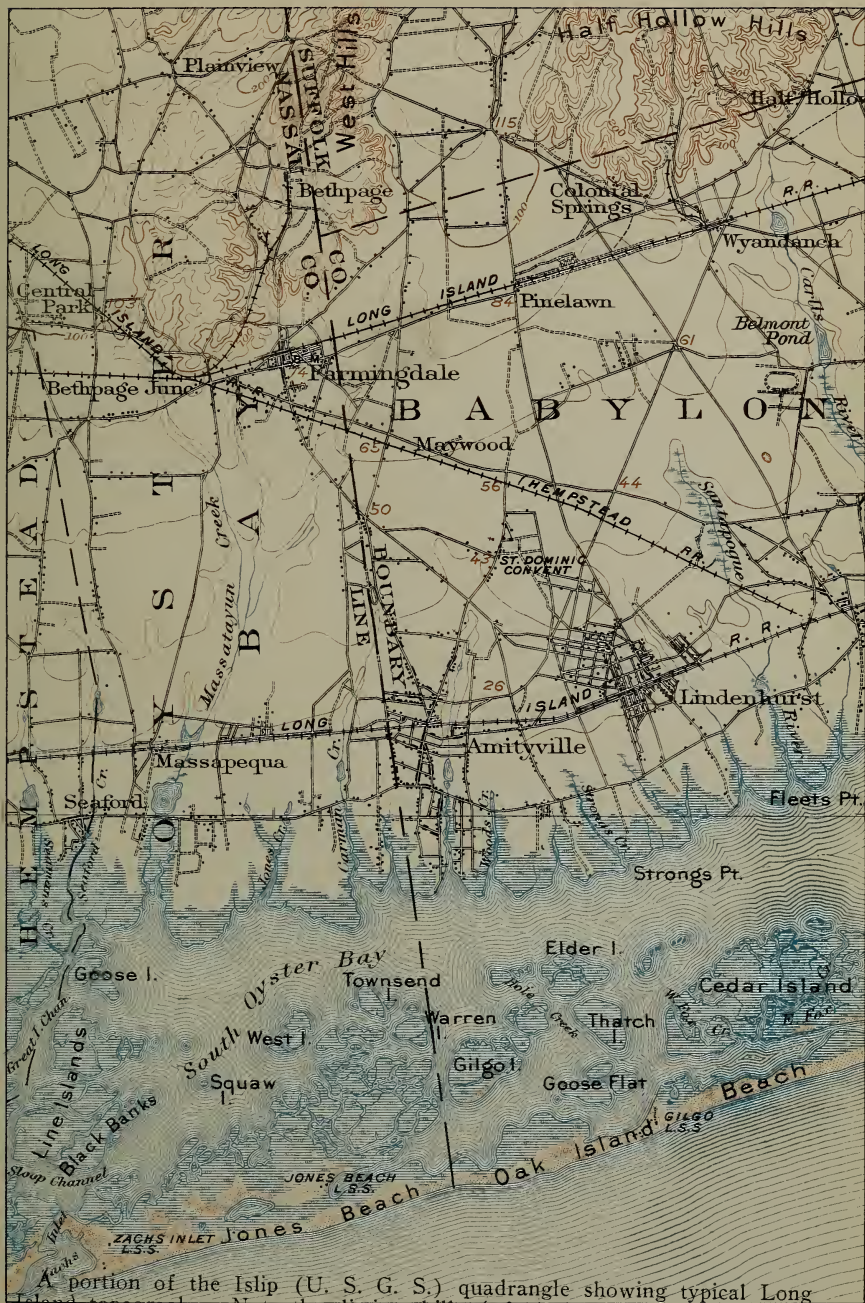
A portion of the Islip (U. S. G. S.) quadrangle showing typical Long Island topography. Note the distinct hills (of glacial morainic origin) on the north, the perfect plain only very slightly stream-dissected and with very gentle seaward slope, and the long beach (built by wave action) inclosing the shallow bay with its many swampy islands. Scale, about 2 miles to the inch.
