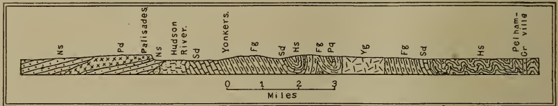
FIG. 20 Detailed section running west-northwest through Pelhamville, Yonkers and the Palisades in southeastern New York, showing the intense folding of Taconic age, the granite dikes, and the relation of the Palisade lava to the other formations. Fg=Fordham fineiss (Precambric); Pq=Poughquag quartzite (Cambric); Sd=Stockbridge dolomite (Cambro-Ordovician); Hs=Hudson schist (Ordovician); Yg=Yonkers gneiss; Gr=granite dike; Ns=Newark sandstone (Jura-Trias); Pd=Palisade diabase or lava (Triassic).
