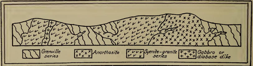
FIG. 12 Generalized section showing the relations of the most common Precambric (Adirondack) rocks to each other and how their relative ages are determined.
