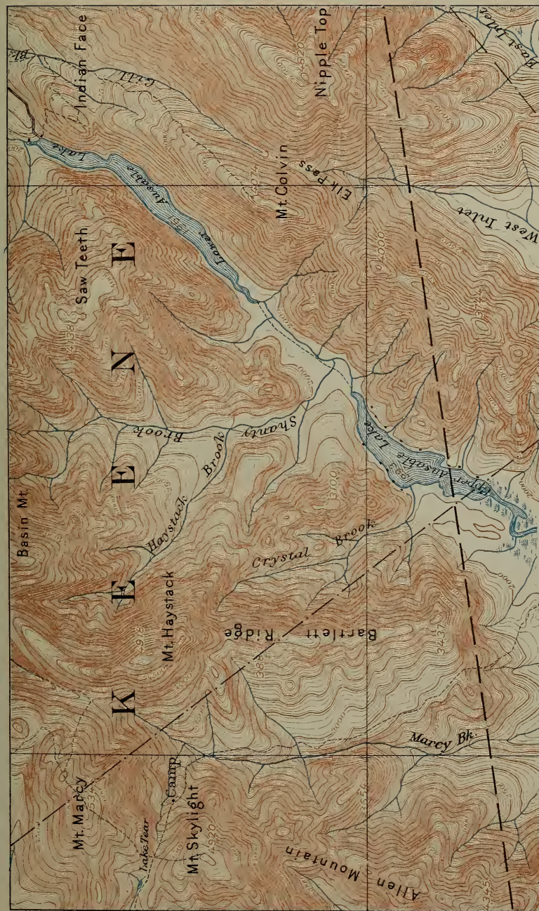
The highest and most rugged Adirondack topography, as represented by a portion of the Mt Marcy (U. S. G. S.) quadrangle. One of the northeast-southwest ridges so common in the eastern Adirondacks is shown just east of the lakes. The rocks are nearly all of plutonic igneous origin (anorthosite). Scale, about 1 mile to the inch. Those who are not familiar with the topographic map and its interpretation should refer to the explanation in the appendix.
