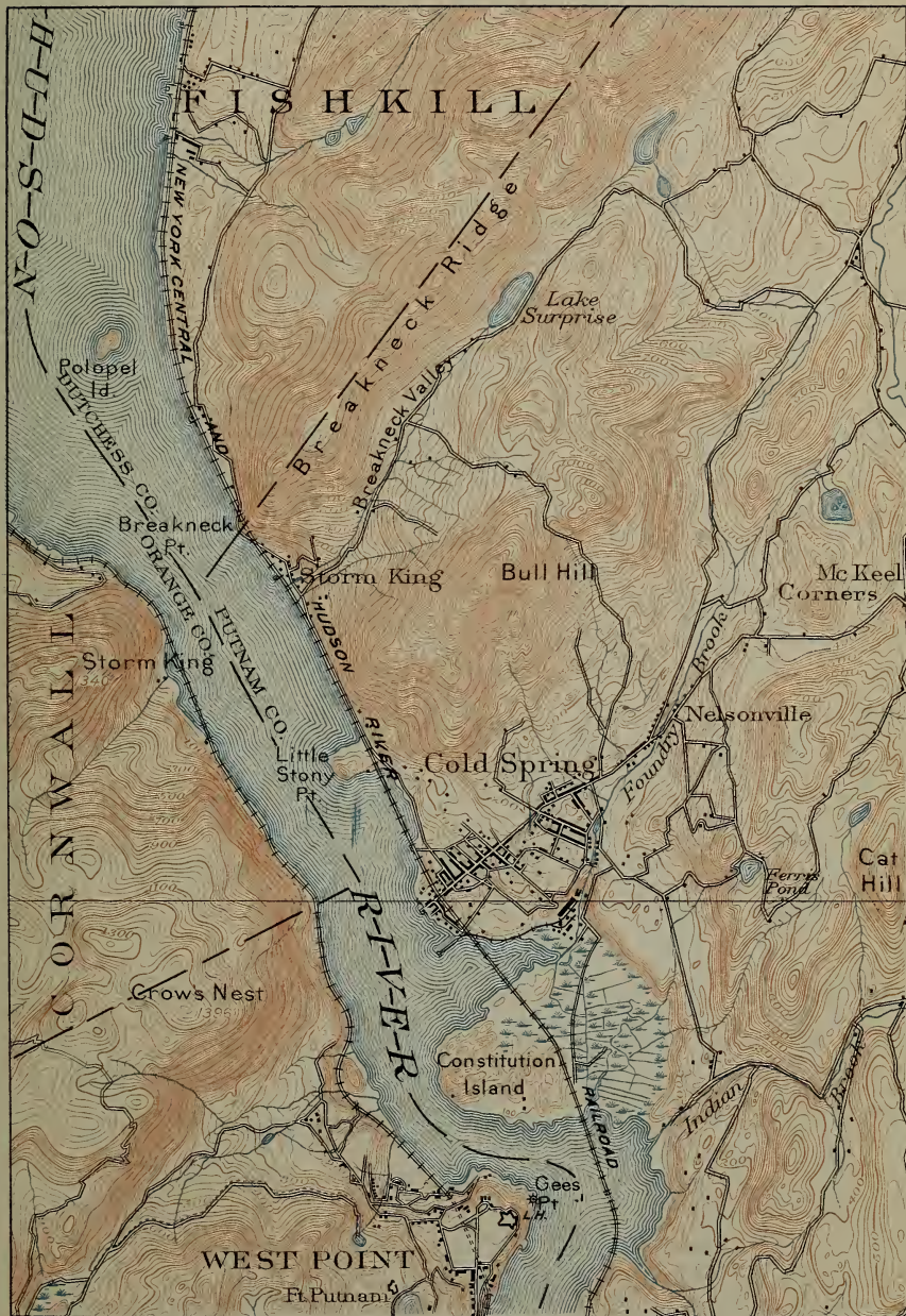
A portion of the West Point (U. S. G. S.) contour map, illustrating the topography of the Highlands of the Hudson. The river here flows through a deep, narrow gorge which has been cut through the northeast-southwest ridges of very hard Precambrian rock. The sides of the gorge rise abruptly from the river to heights of 1200 or 1400 feet, while the rock bottom of the gorge is hundreds of feet below the river level. Scale, about 1 mile to the inch.
