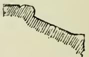
^ FIG. 152.— Jamb of a Door found at Athens —IXth Century (after Castel- lazzi).
