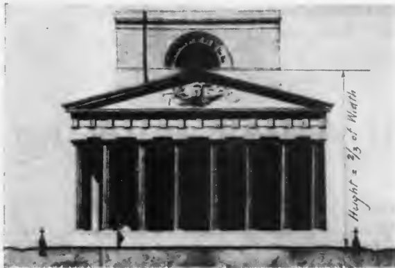
Fig. 1—Design for the Bank of the United States, Philadelphia, showing the proper proportions for a classical façade. Benjamin H. Latrobe was the architect
