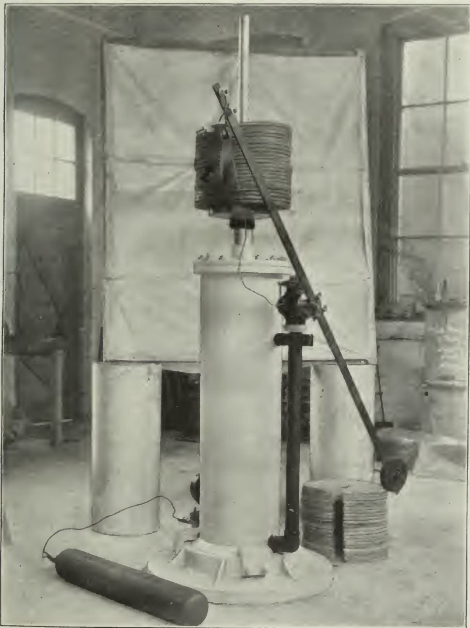
C. APPARATUS FOR IGNITING COAL DUST BY GAS FLAME, ALTOFTS EXPERIMENTAL GALLERY.
