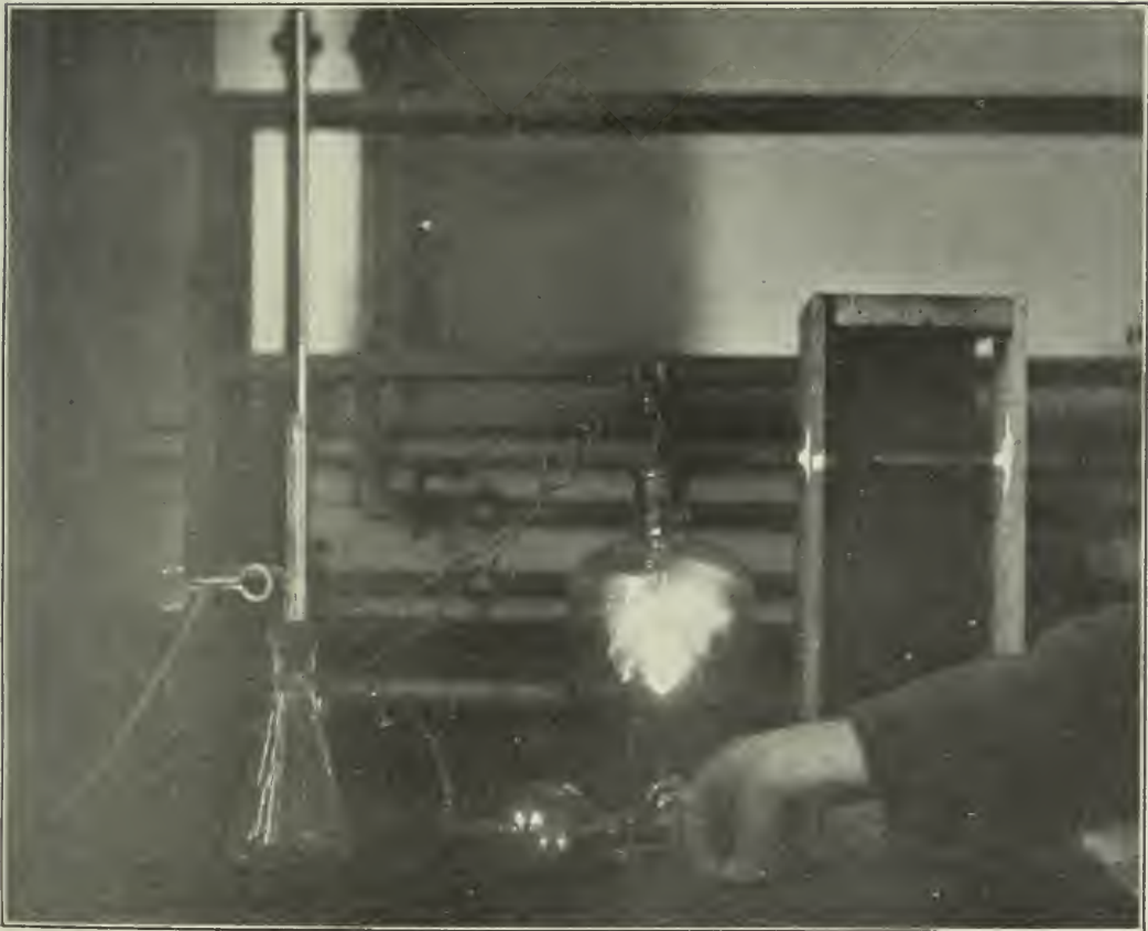
B. APPARATUS USED AT PITTSBURG, SHOWING IGNITION OF DUST.
