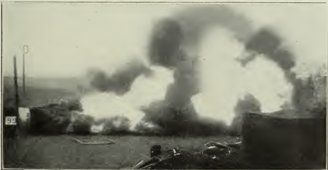
C. EXPERIMENT 99 AT ALTOFTS GALLERY, SHOWING FLAME AND SMOKE ISSUING TO A DISTANCE OF 160 FEET FROM EXPLOSION OF 375 FEET OF COAL-DUST ZONE.
