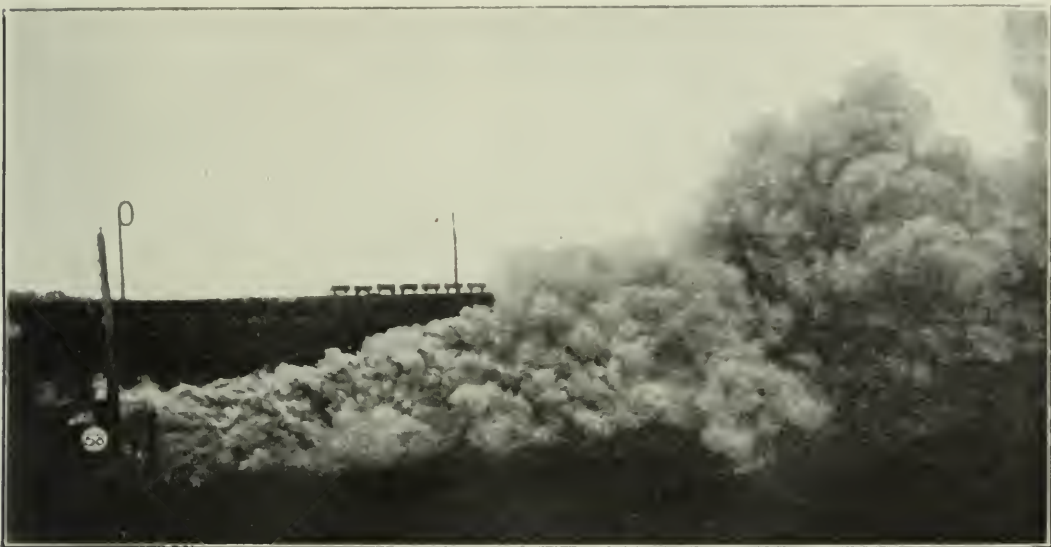
B. EXPERIMENT 58 AT ALTOFTS GALLERY, SHOWING STONE DUST AND SMOKE ISSUING FROM GALLERY AS THE RESULT OF AN EXPLOSION OF THE 275-FOOT COAL-DUST ZONE.
