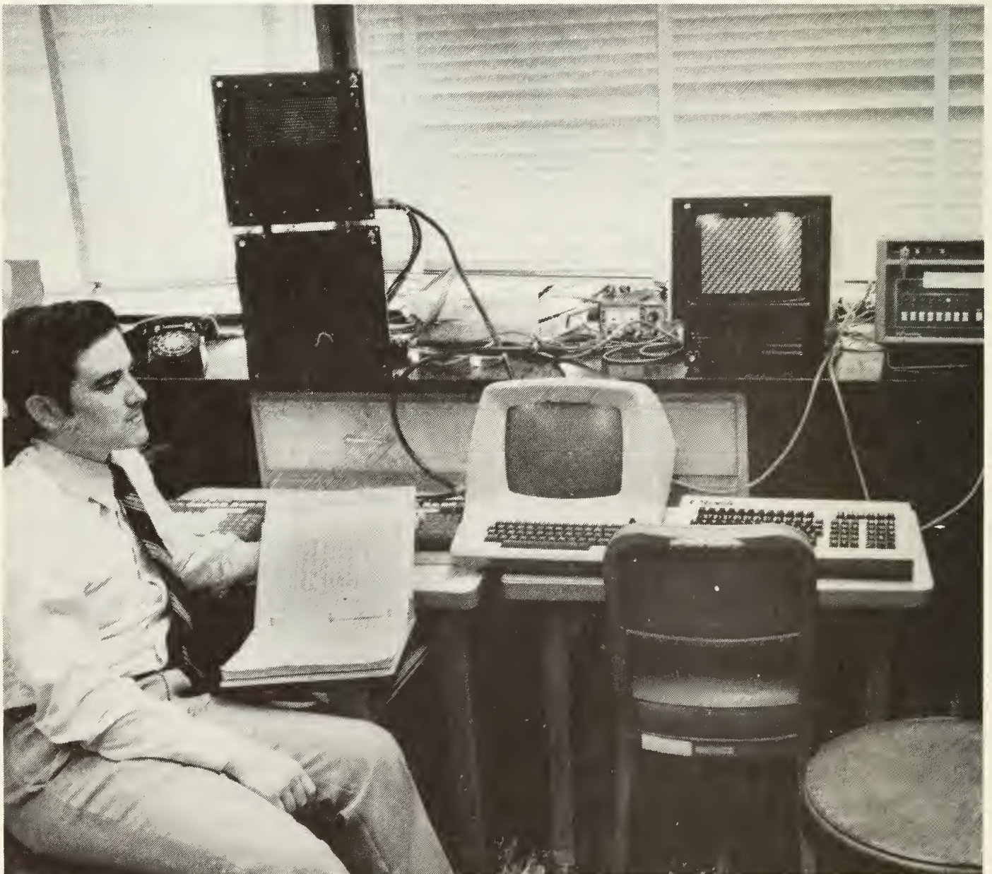
Set-up for shipboard tactical position display that uses a microcomputer driven plasma display
