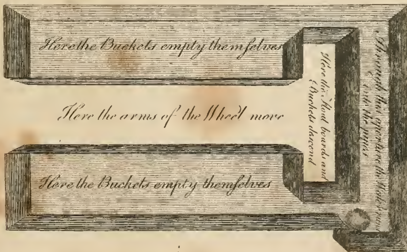
Sketch of the manner in which the Water is filled from the Troughs into the Buckets.
