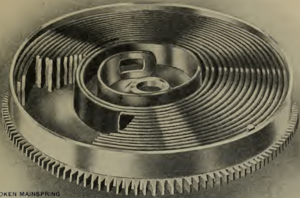
BROKEN MAINSPRING IN A WATCH BARREL
