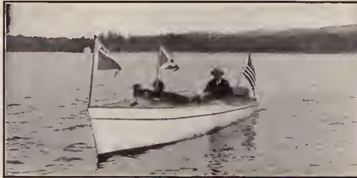
No. 99.—22-ft. x 4 ft. 2 in. Highspeed runabout, V bottom; Leighton 4-cyl., 50 h.p. motor. Bosch ignition; fine condition. Speed 27 miles. Bargain. Please mention MOTOR BOATING.
