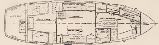
Interior arrangement similar to the Margo II. One double stateroom, sleeping two in beds. Saloon with drop table and sleeping accommodations for four. Galley, engine-room and crew's quarters in combination.
