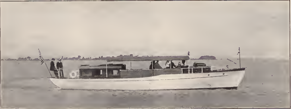
50' x 9' x 3'6" Florida day cruiser ZUMBROTA, 32-37 H.P. Standard Motor. Speed 13 miles. Mahogany finish. Crew's quarters, motor space, large cockpit, main cabin, galley, and two toilets. Sleeps four comfortably. Boat in Florida. Write for particulars.
