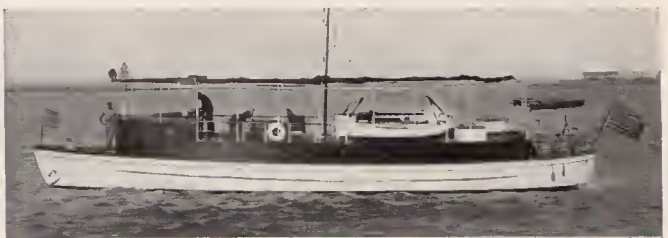
Colonel, which is in service with the U. S. Engineers at Galveston, Texas. She is powered with two four-cylinder 40 h.p. Lamb engines.
