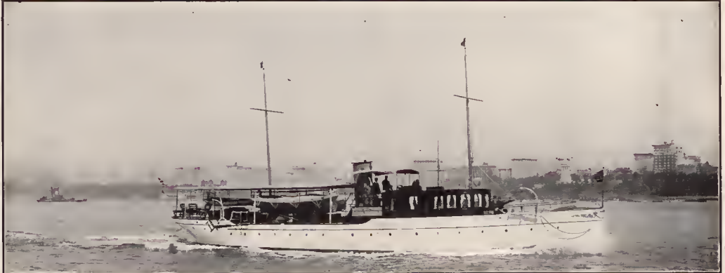
No. 1820.—For Sale or Charter.—Modern, twin-screw cruising power yacht, 98 ft. x 16 ft. x 4 ft. Built 1911 from our designs. Speed 14-16 miles; two 100-125 h.p. 6-cylinder air-starting Standard engines. Large accommodation, including five staterooms and two bathrooms aft; dining saloon and galley forward. Price attractive. Cox & Stevens, 15 William St., New York City.
