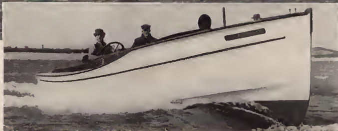
Seemego is a Hand V-bottom boat modeled after Piute IV, but having a refinement in line details which gives her a better speed with the same power.
