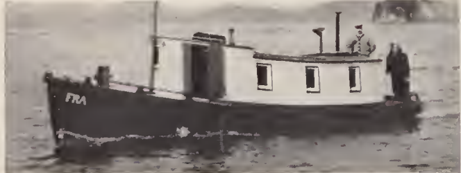
The 34-foot Fra, owned at Hoonah, Alaska. She is powered with a two-cylinder, 8-10 Sterling engine, giving her a speed of 10 m.p.h. it is claimed.
