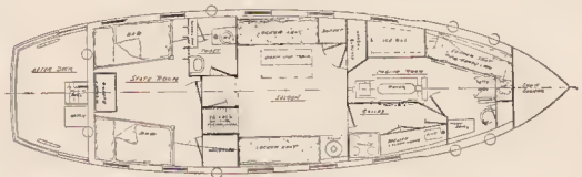
Plan the same as arrangement No. 1, except that galley is separated from engine-room and crew's quarters; owner's toilet being moved aft.
