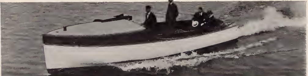
Reeling of the required speed of 15 miles on her trial trip in Camden Harbor. Subsequent to the taking of this picture the cruiser was fitted with six port lights, cockpit awning, and a sheathing of yellow metal six inches above the waterline.
