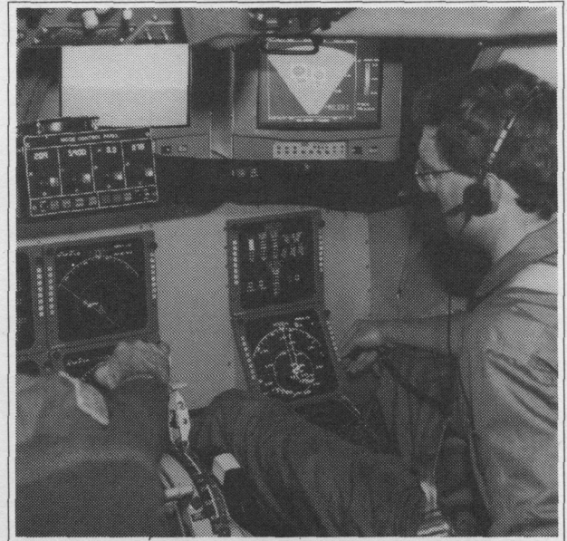
The cockpit of Langley’s 737 research aircraft displays windshear data prior to penetrating a microburst.
