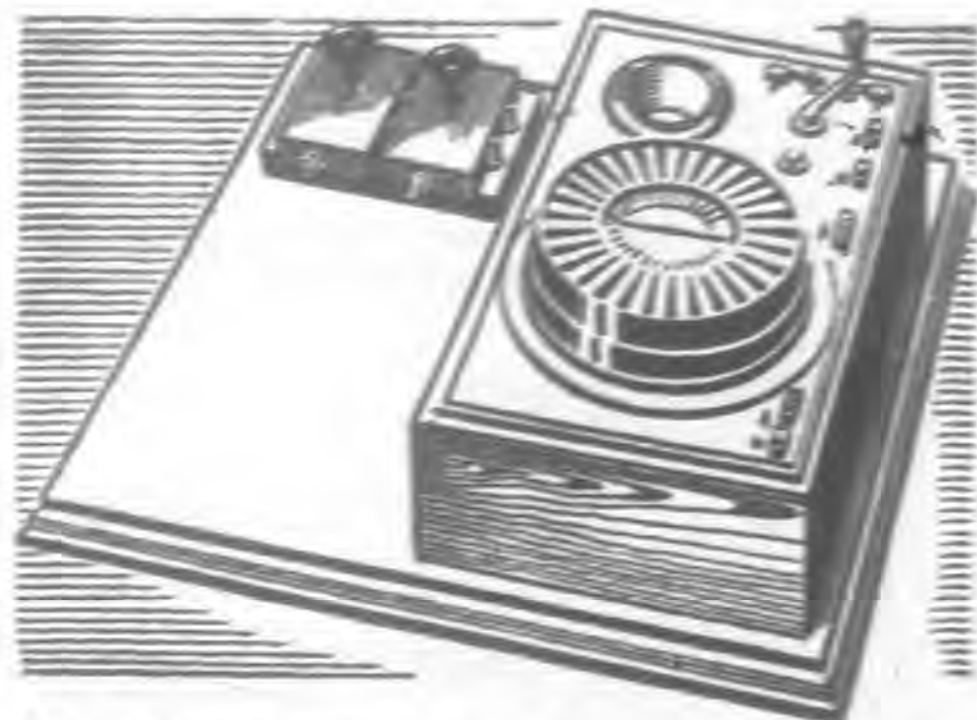
Model of the first needle-telegraph, invented by Siemens and constructed by his collaborator Halske.
