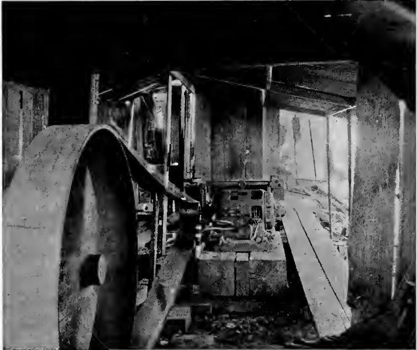
FIG. 53. Westinghouse motor belted for drilling.
