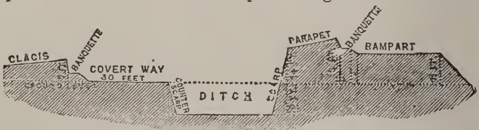
Vertical Section of Defense-works.
