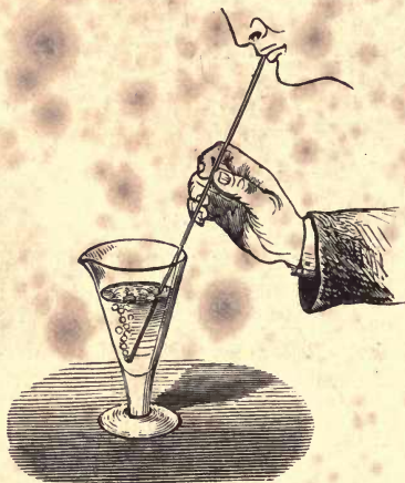
FIG. 32.—Carbonic di-oxide from the lungs passed into Lime-water ( \text{Ca O}_2 \text{ H}_2 ).
