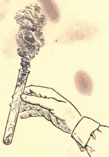
FIG. 43.—Mercury dissolving in Nitric acid.
