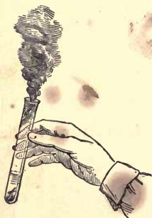
FIG. 35.—Silver coin dissolving in Nitric acid.
