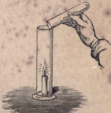
FIG. 31.—Pouring Carbon di-oxide from one vessel to another to extinguish a burning candle.
