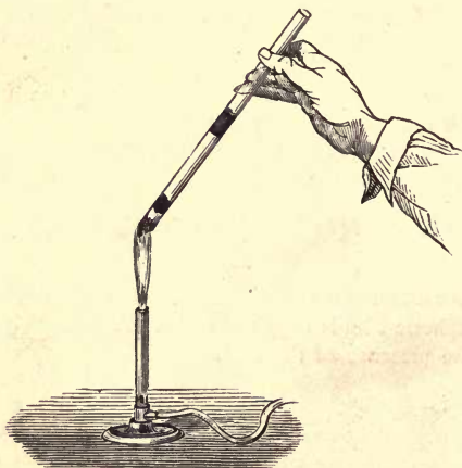
FIG. 27.—Arsenious oxide detected by heated charcoal.
