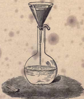
FIG. 30.—Indigo solution decolorized by filtering through animal charcoal.
