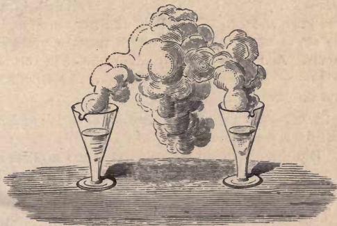
FIG. 23.—Ammonia-gas and Chlorohydric-gas meeting in the air and forming Ammonic chloride.
