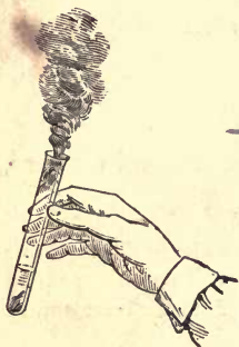
FIG. 24.—Nitric acid dissolving Copper.
