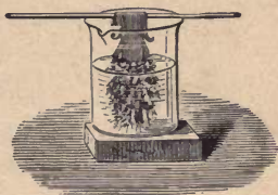
FIG. 40.—The Lead-tree precipitated by metallic Zinc.
