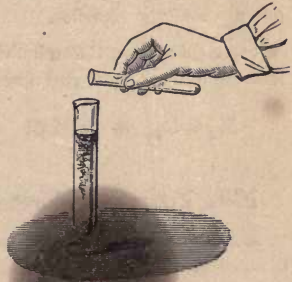
FIG. 25.—Making a precipitate of Argentic chloride.
