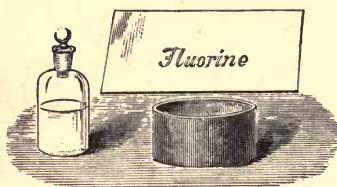
FIG. 10.—Etching glass by means of gaseous Fluohydric acid.
