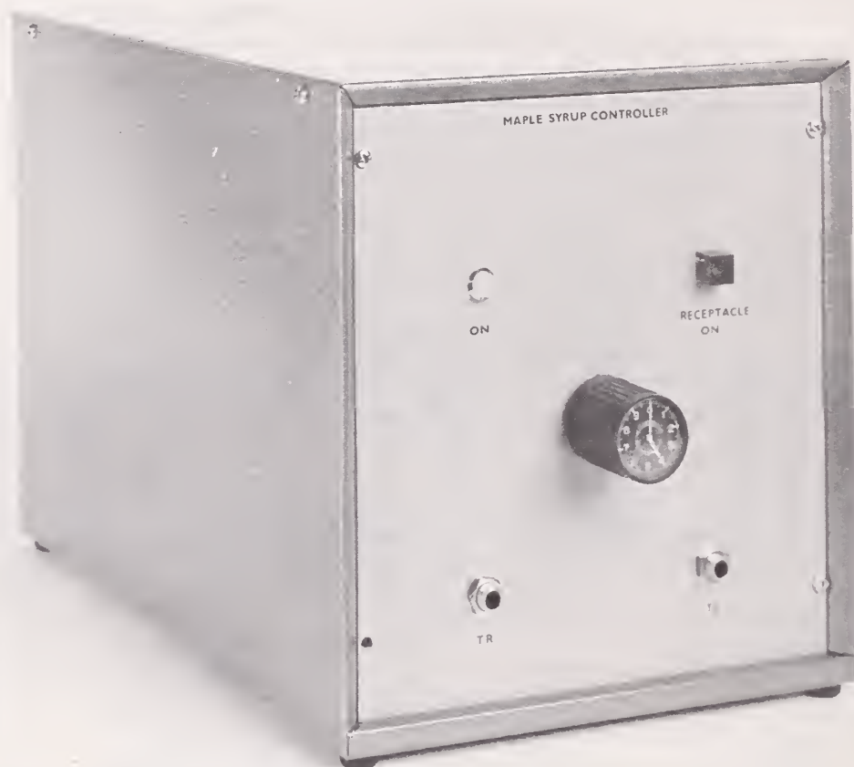
Figure 6. --Photograph of automatic controller using operational amplifier
