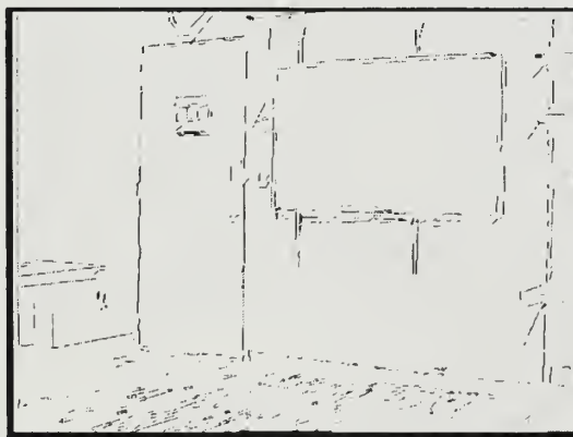
Figure 30. Line segment extraction via findedge implementation. C_3 = 0.1 , C_4 = 7 pixels, C_5 = 7.0 .
