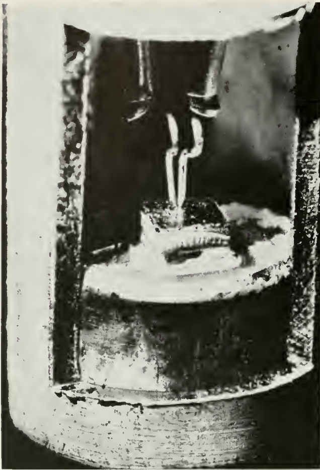
A portion of the "cartridge" casing of a point-contact transistor has been cut away to show, magnified, the two points on the germanium surface
