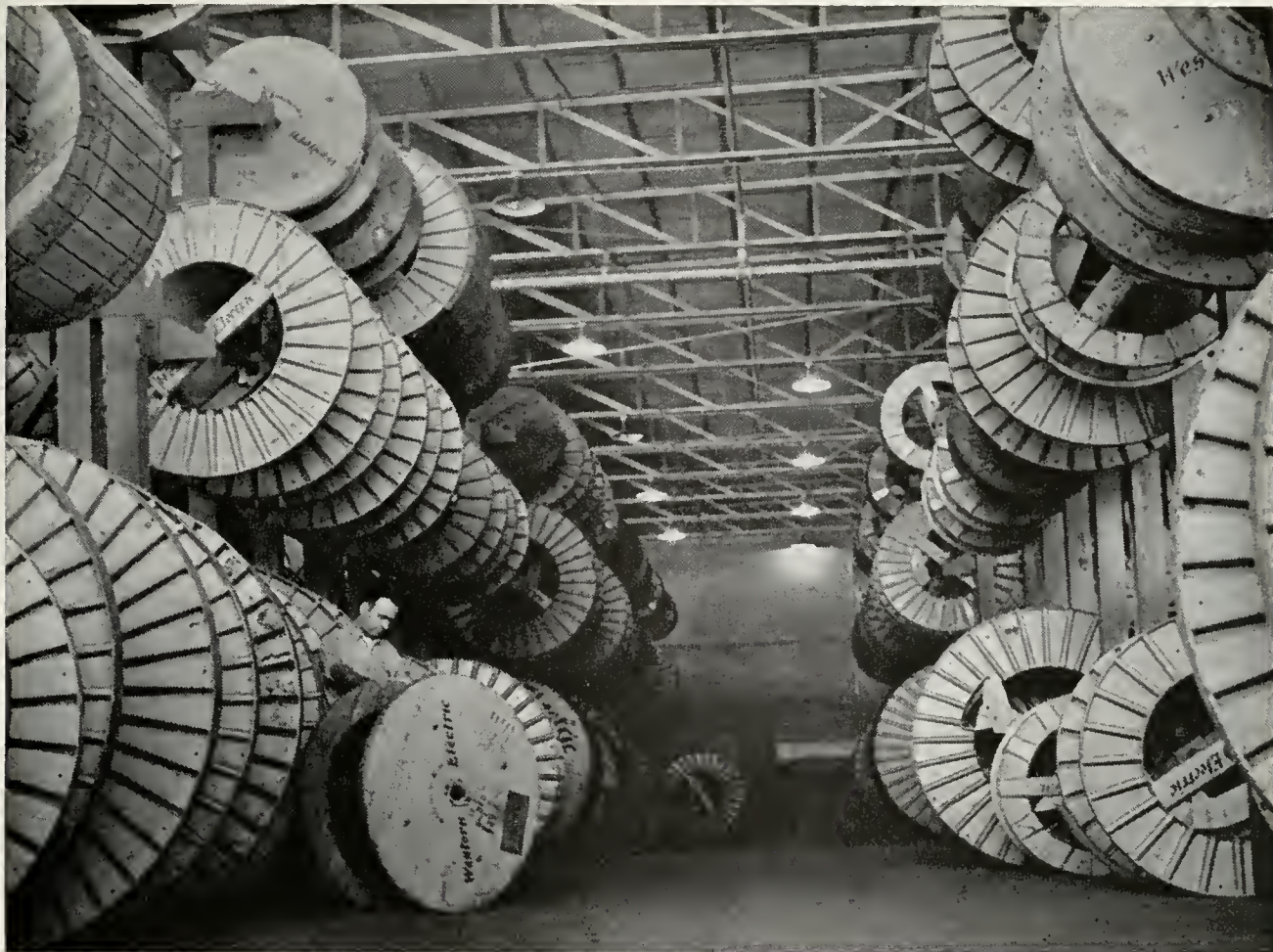
Reels of telephone cables three tiers high show space conservation in Western's distributing houses. A new cable-measuring machine pulls cable from overhead reels and cuts it to exact length
