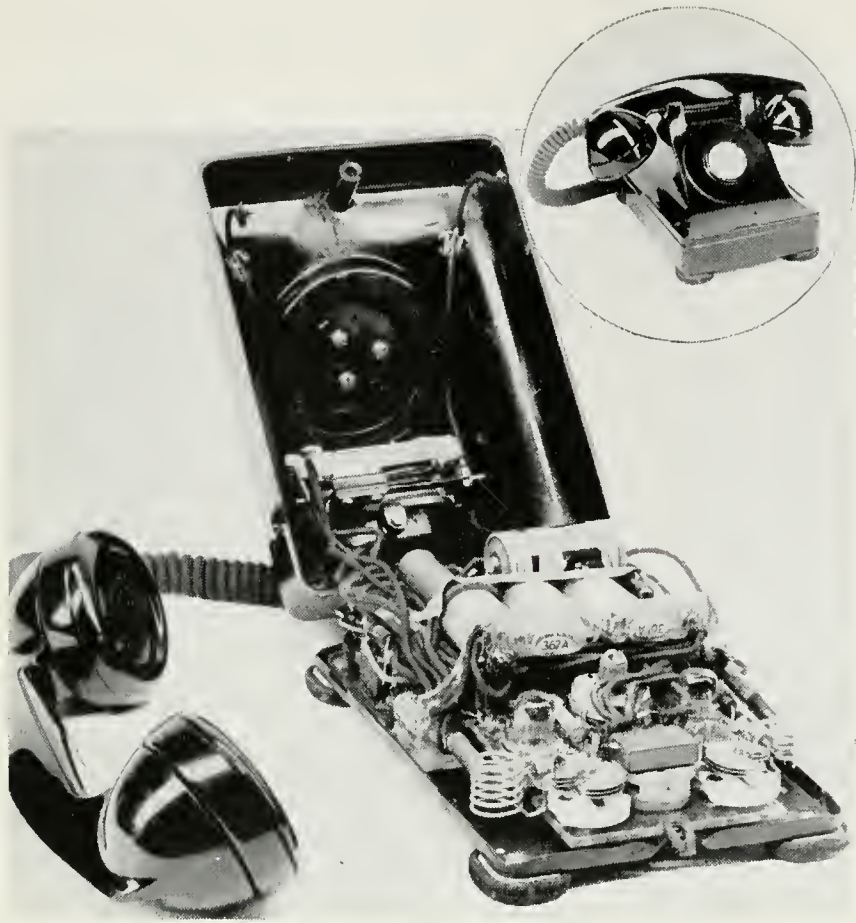
"Wireless Telephone": an experimental set containing a very-short-range radio, to eliminate the customary telephone cord
