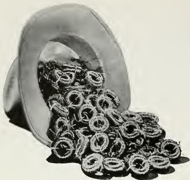
Loading coils by the hatful with cores of Permalloy. Two and one-half times as many coils are produced today per pound of nickel as in 1940
