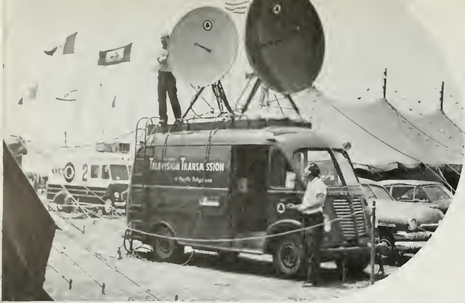
These mobile transmitters beamed television signals to 5,000-foot Mt. Wilson, 48 miles away, and thence into regular television channels. Below: Telephones were essential to the administration of the huge enterprise. Commissary headquarters, for example, used three telephones to dispatch its trucks
