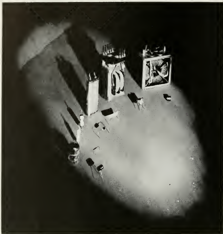
Miniature apparatus components have been developed to work with the transistor. The transistor itself is small compared to the smallest vacuum tubes. Resistors, capacitors, transformers, inductors are all correspondingly smaller than their counterparts used with vacuum tubes
