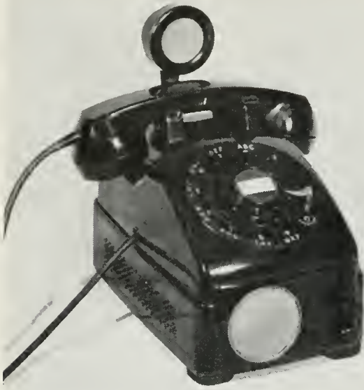
An experimental "distant talking" set: you would speak to it and listen to it without holding or switching anything
