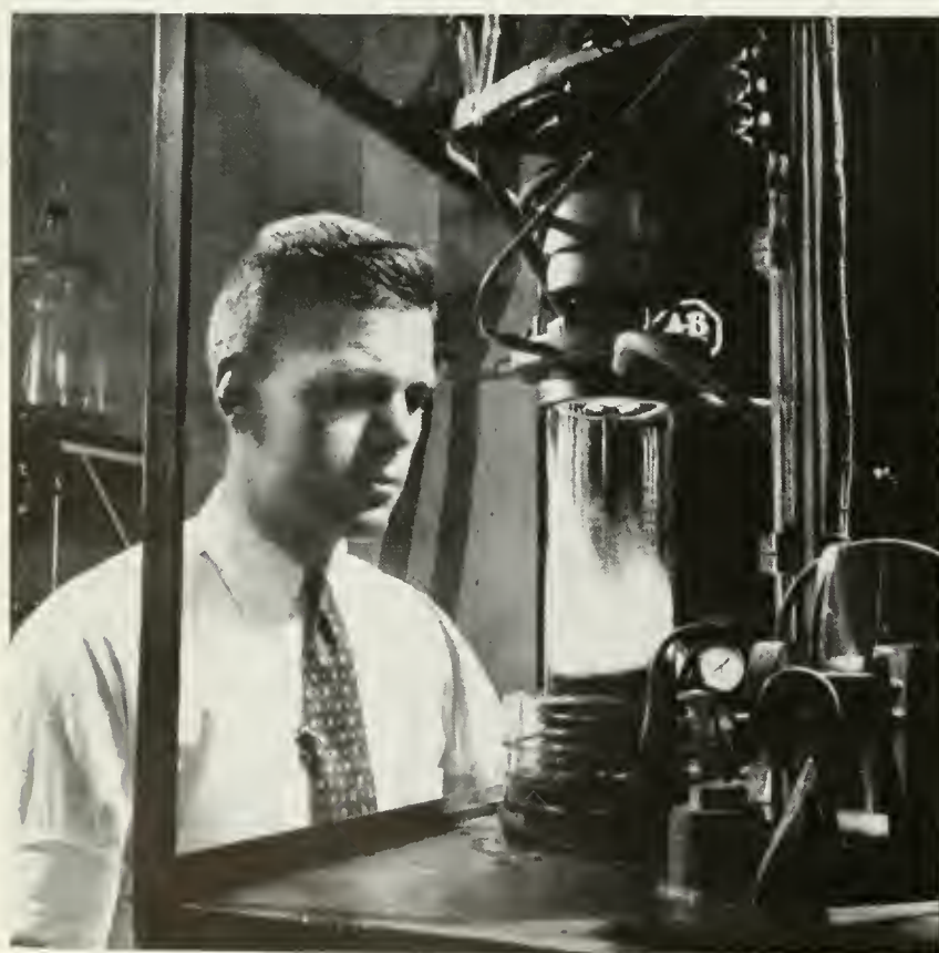
Silicon, another important semiconductor, is purified and grown in "single crystal" form in this apparatus by F. Buehler
