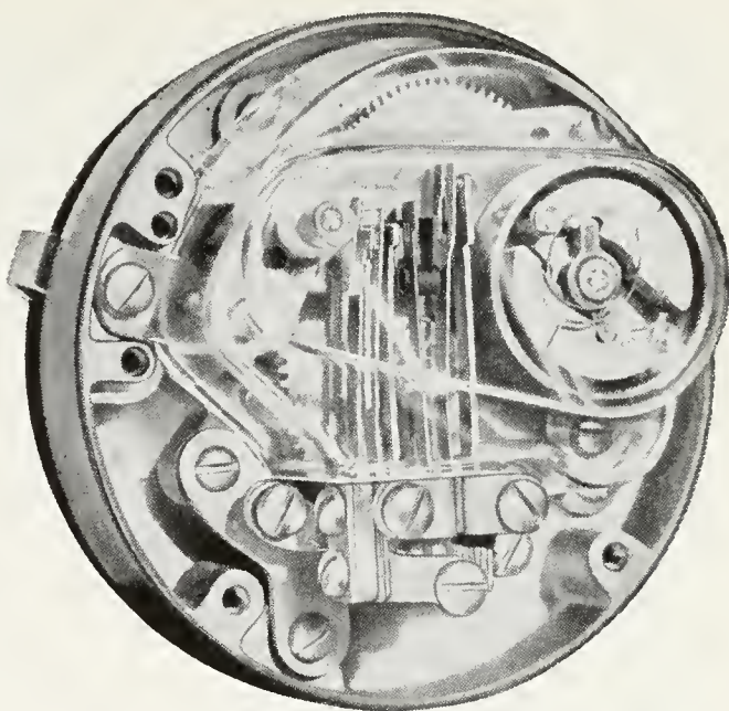
A telephone dial mechanism—viewed from underneath. Four of the six contact springs, as well as three parts of the governor, are made of nickel silver
