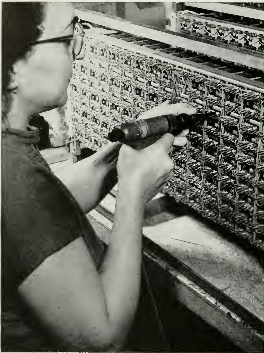
"Shooting" wire connections onto terminals eliminates pliers, soldering iron, solder, and many motions in making six hundred million electrical connections a year in Western Electric factories
