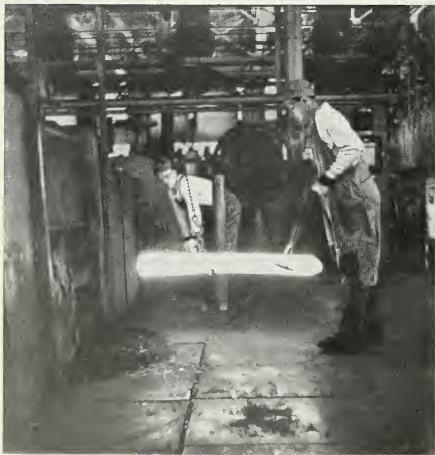
A white-hot ingot of Permalloy being guided into a Western Electric hot-rolling mill
