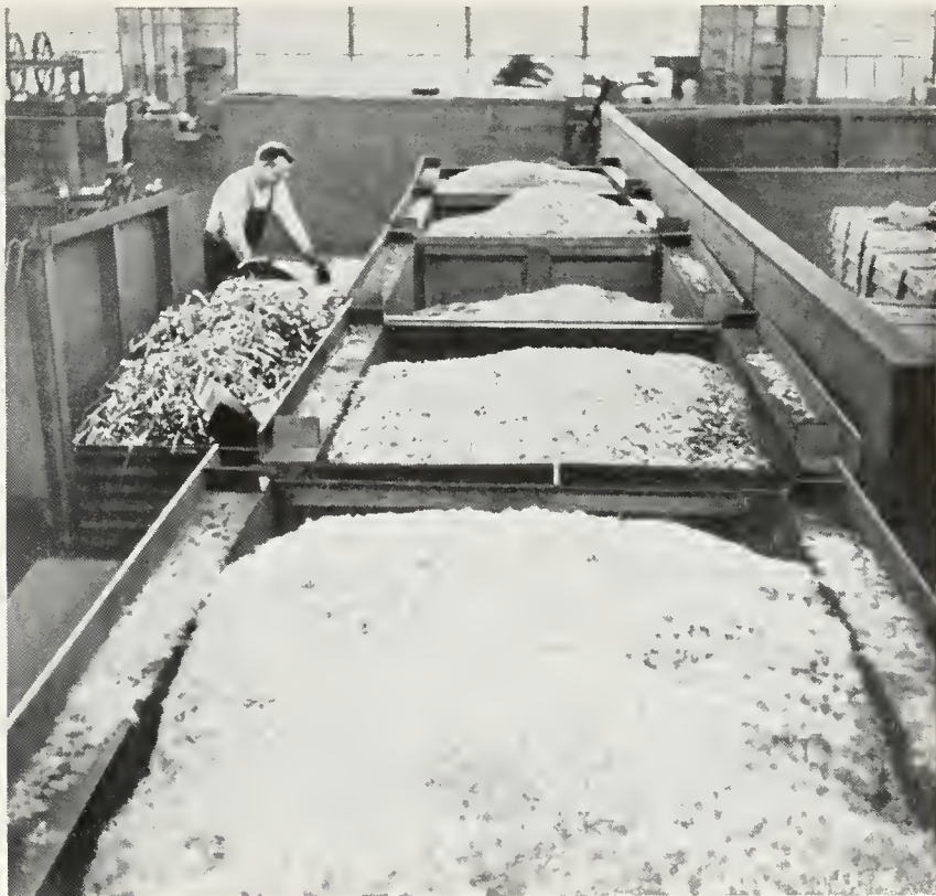
Metal scrap like this is processed in Western Electric's metals mill. Nearly one-third of the nickel content of all nickel silver and magnetic alloys used currently by Western Electric is recovered from its own scrap
