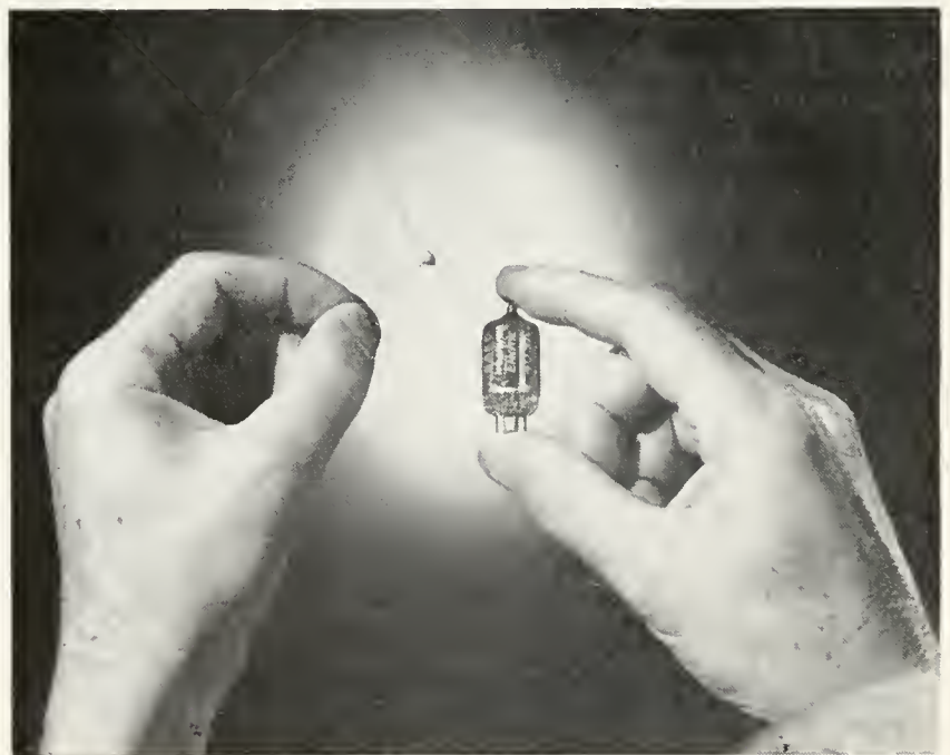
The tiny plastic bead of the transistor contrasts with the famed "peanut" (6AK5) vacuum tube
