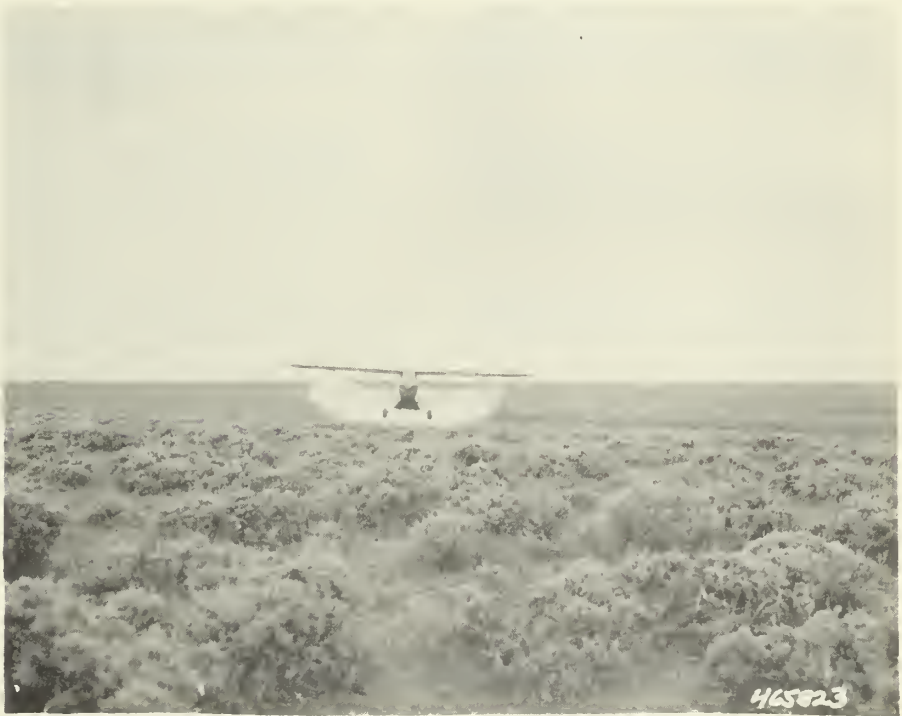
Figure 2.--The airplane equipment sprayed a 50-foot swath at 90 miles per hour. Height of flight was from 2 to 10 feet.
