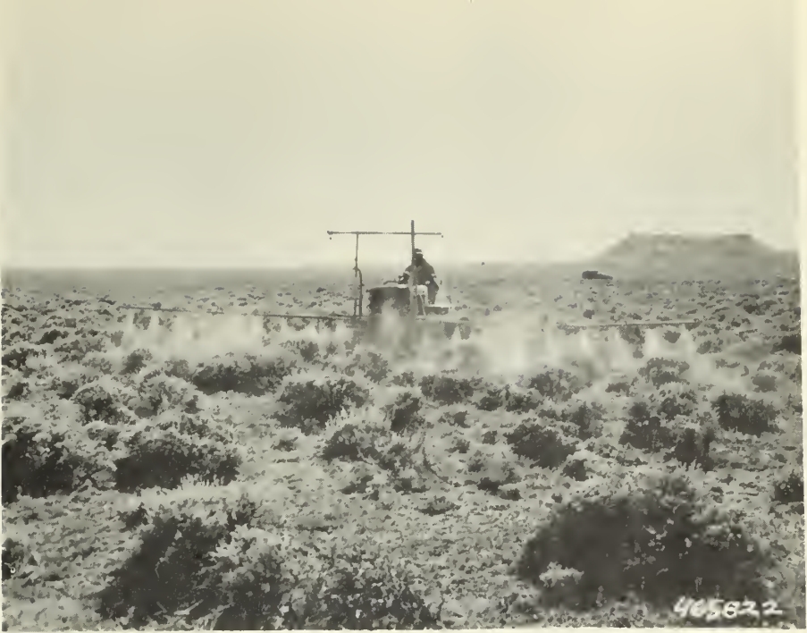
Figure 1.--This tractor-mounted spraying equipment covered a 30-foot swath at 3 miles per hour. The spray tank is behind the operator.
