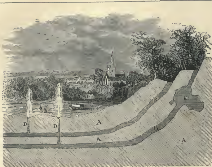
Artesian Wells:—A, A, A, Strata impervious to Water,—B, B, Seams or Strata in which Subterranean Streams flow; C, Subterranean Reservoir filled with Water;—D, D, Borings in the Ground or Rock, called Artesian Wells.
