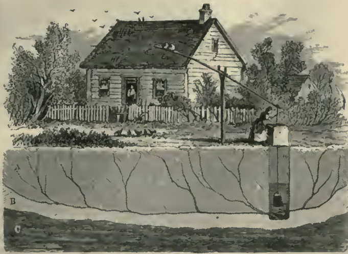
Section of the Ground or Rock, showing how Wells are supplied. A. The Part through which the Rain Water percolates. C. Rock or Clay impervious to Water B. Seam or Stratum in which the Water passes.
