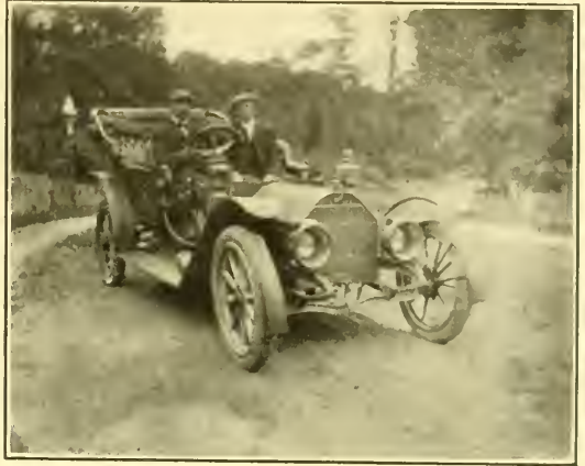
Fenders in their Elevated Position
