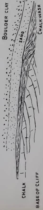
Shewing the true slope of the surface of chalk on which the Chalk Wash rests.
