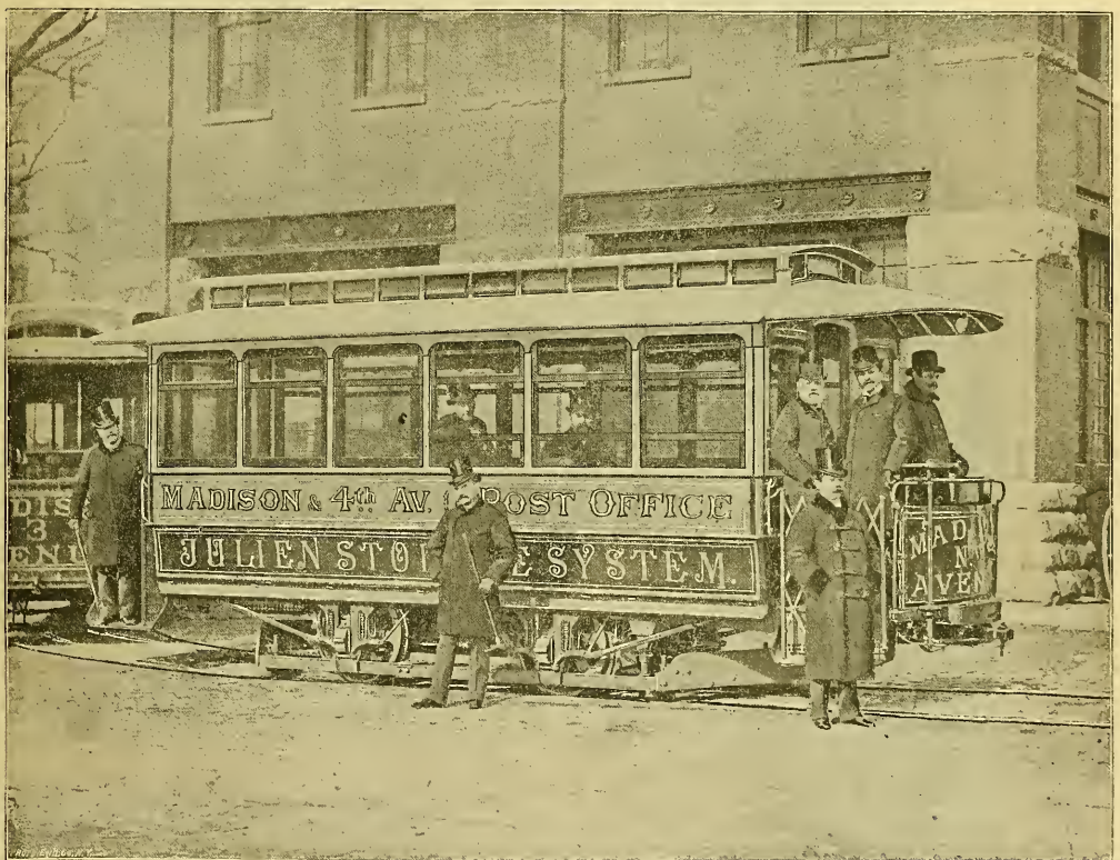
STREET-CAR DRIVEN BY JULIEN STORAGE-BATTERIES.
