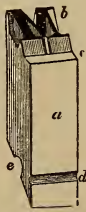
Metal Type. a, the body; b, face; c, shoulder; d, nick; e, groove.
