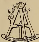
Hadley's Quadrant. t , index glass; h , horizon glass; s , sight.
