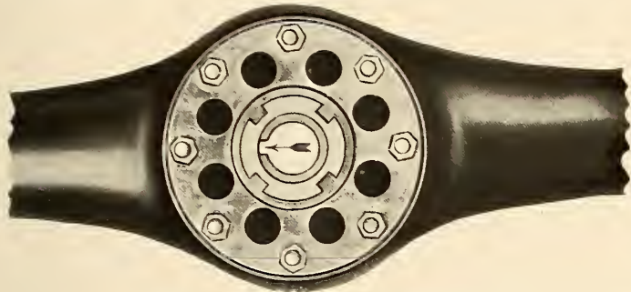
Location of keyway in propeller hub
