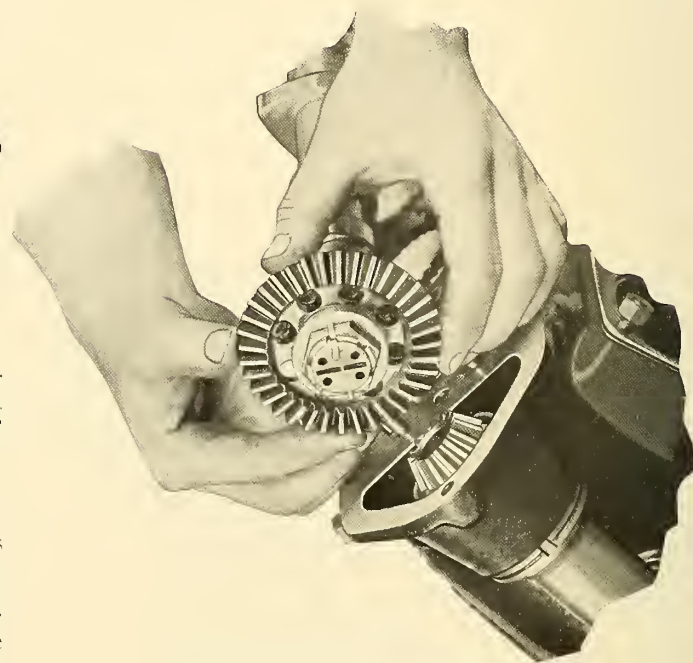
Changing meshing of camshaft gear
