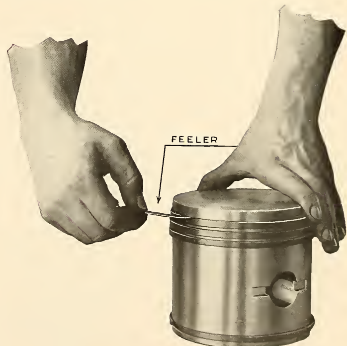
Checking side clearance on piston rings
