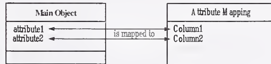
Fig. 2 Mapping attributes of an XML Element to the columns of its corresponding RDB table
