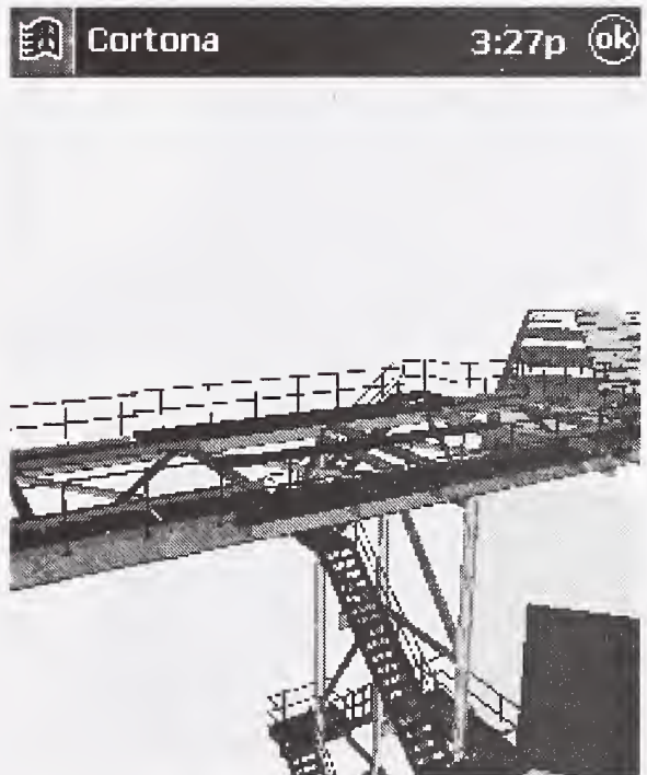
Figure 2. Steel support structure for the NIST ECS.
