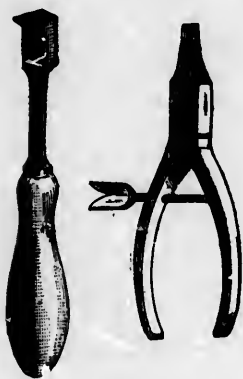
FIG. 11. INSTRUMENT USED IN SAXONY TO OPEN MUSSELS WITHOUT KILLING THEM.
