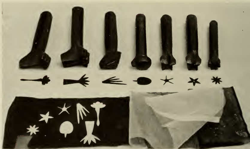
Steel dies may be used for stamping out flower parts, or leaves where the commercial method is used. The material may be waxed cloth, paper or celluloid.
