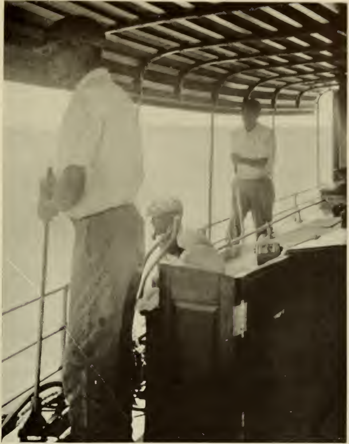
MANNING THE PUMPS ABOARD THE "STANDARD J." Moxie, in the center, acts as tender. It is his duty to watch the divers and to pay out and take in the air-hose as needed
